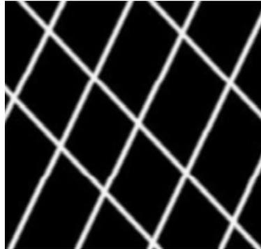
Figure 6.10: Raw test image. The test image is a grid like pattern with an amplitude of 0.5 (127) relative to the maximum possible for 8 bit images (255) against a black background (zero amplitude). Modified after Di-Zang, Sommer, 2007.
