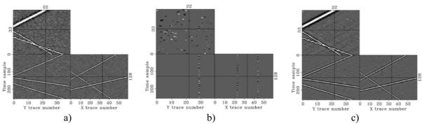
Figure5: a) Original 3D synthetic data b) 90% randomly missing data c) sparse reconstruction result
