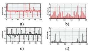
**Figure3:** a) Signal with 80% missing samples. Samples are picked from the decimated signal by factor of 2. c) Sparse reconstruction of a. b, d) Fourier representations of a, c, respectively.
