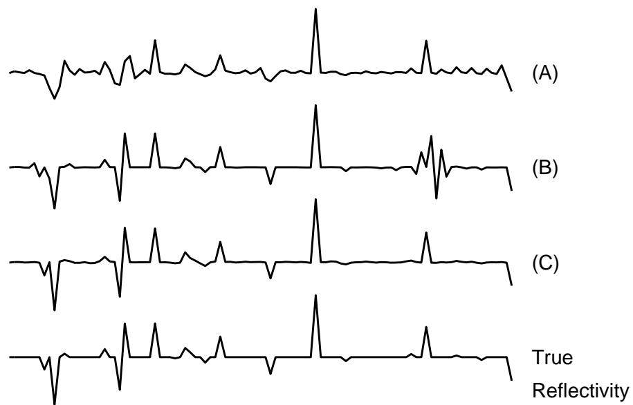
Figure 4.9: The reflectivity series recovered by the exponential (A), Cauchy (B), and modified Cauchy (C) prior distributions, subject to 4 impedance constraints.
