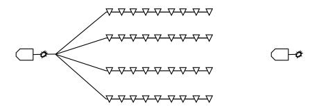
Figure 1.3: Illustration of early marine simultaneous source acquisition with two shots well separated in space (Beasley et al., 1998).
