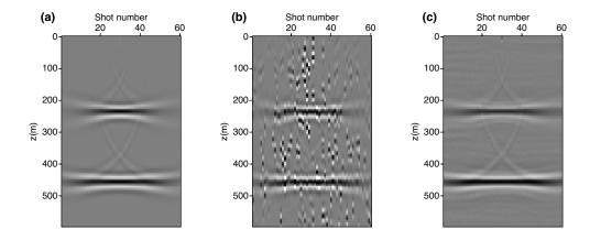
Figure 5.3: Migration results of the two-layer model: a shot-index common image gather (x=600). (a) A shot-index common receiver gather from conventional unblended shot-profile migration; (b) A shot-index common receiver gather from blended shot-profile migration; (c) A shot-index common receiver gather from blended least-squares shot-profile migration.
