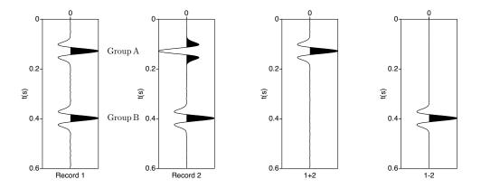
Figure 1.2: Illustration of phase-encoding of dual source simultaneous source acquisition using vibroseis (Meunier, 2011).
