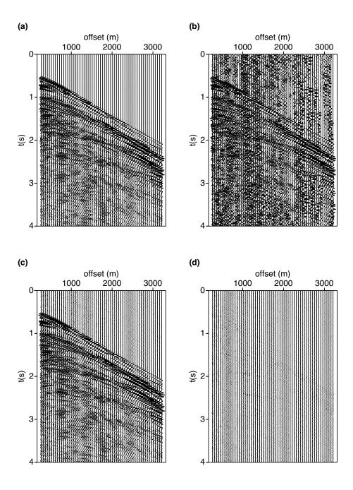
Figure 3.16: Results of simultaneous source separation of a 2D marine line: (a) The real unblended CMP gather. (b) CMP gather sorted from Pseudo-deblended data. (c) Deblended results via the proposed algorithm. (d) Differences between (a) and (c).In this example, the signal-to-noise ratio after separation is 14.2dB.
