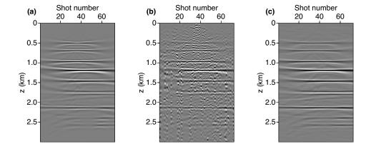
Figure 5.9: Migration results for SAIG velocity model: a shot-index common image gather (x=2.5km) (a) A shot-index common receiver gather from conventional unblended shot-profile migration; (b) A shot-index common receiver gather from blended shot-profile migration; (c) A shot-index common receiver gather from blended least-squares shot-profile migration.
