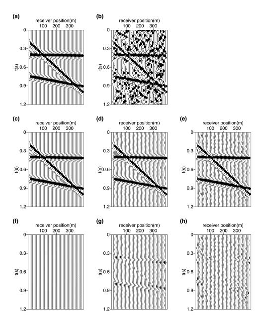
Figure 4.2: Comparisons of deblending results for numerically blended synthetic data with linear events. (a) The original unblended synthetic data. (b) Pseudodeblended gather. (c) Deblending result with the proposed iterative rank reduction method. (d) Deblending result using iterative f-x deconvolution. (e) Deblending results using iterative f-k domain thresholding. (f) Difference section between a and c. (g) Difference section between a and d. (h) Difference section between a and e
