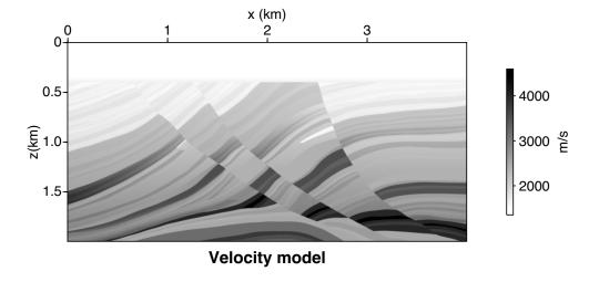
Figure 5.13: The Acoustic Marmousi2 model.
