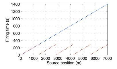
Figure 4.4: Spatial and temporal distribution of firing times for conventional seismic acquisition (Blue) and 2D simultaneous source acquisition. The multi-vessel scenario is portrayed in red. In each round, 5 sources fire with small random time delays. The spatial distance between sources are fixed in each round.
