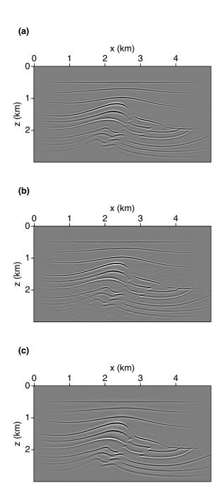
Figure 5.11: Migration results for SAIG velocity model: stacked image (a) Stacked image from conventional unblended shot-profile migration; (b) Stacked image from the blended shot-profile migration; (c) Stacked image from the blended least-squares shot-profile migration.
