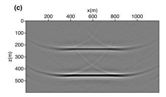
Figure 5.4: Migration results of the two-layer model: partial image for shot 30. (a) A partial image from conventional unblended shot-profile migration; (b) A partial image from the blended shot-profile migration; (c) A partial image from the blended least-squares shot-profile migration.
