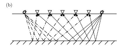
Figure 1.1: Comparison of the acquisition geometry between (a) conventional seismic acquisition, and (b) simultaneous source acquisition.
