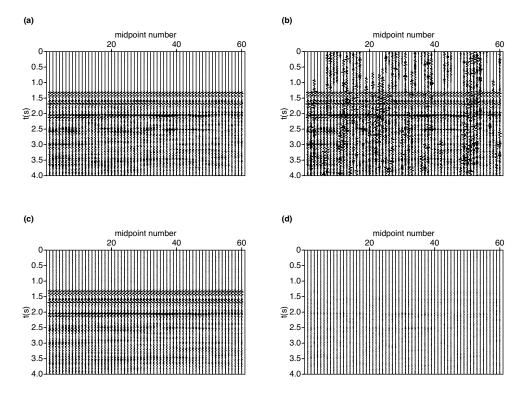
Figure C.3: Deblending via RPCA. (a) The unblended common offset gather. (b) Pseudo-deblended common offset gather. (c) Common offset gather after RPCA de-noising. (d) Differences between (a) and (c).
