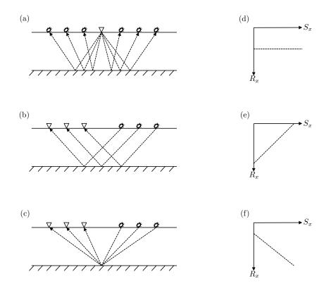
Figure 1.4: Illustration of gathers with each trace correspoding to a different source location. The figures on the left shows the source and receiver pairs of (a) common receiver, (b) common offset, and (c) common midpoint gathers. The figures on the right shows the illustration of a (d) common receiver, (e) a common offset, and (f) a common midpoint gather in 2D seismic acquisition.
