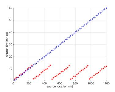
Figure 5.1: Distribution of firing times for simultaneous source acquisition (red) compared to conventional acquisition (blue). In this example about 75% of acquisition time is saved by source blending. The computational efficiency exhibits a similar pattern for the proposed least squares migration.
