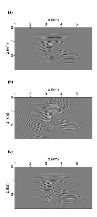
Figure 5.10: Migration results for SAIG velocity model: a partial image for a shot  $(S_x = 2.5km)$ . (a) A partial image from conventional unblended shot-profile migration; (b) A partial image from the blended shot-profile migration; (c) A partial image from the blended least-squares shot-profile migration.
