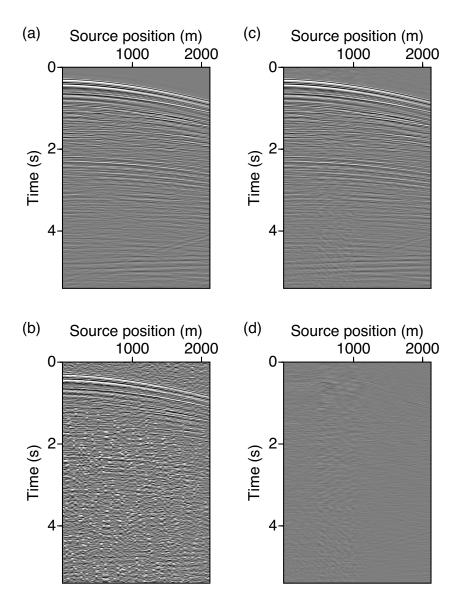
Figure 4.16: Results of deblending for a common receiver gather using optimal source fire time delays. (a) The original common receiver gather from the Gulf of Mexico dataset. (b) Pseudo-deblended common receiver gather (c) Deblended common receiver gather with iterative SSA filtering (d) Difference section between original and deblended data.
