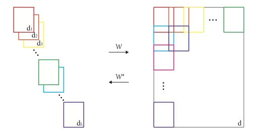
Figure 4.1: The windowing operator and its adjoint operator. The windowing operator  $\mathcal{W}$  extracts small patches of data from an entire gather. The adjoint operator  $\mathcal{W}^*$  combines all the processed small patches back into a gather. A Gaussian taper is used to combine areas with overlap.
