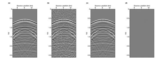
Figure 3.8: Results of simultaneous source separation in common receiver domain when STR equals to 2: (a) The real unblended common receiver gather (centre receiver). (b) Pseudo-deblended common receiver gather. (c) Deblended common receiver gather after 20 iterations. (d) Differences between (a) and (c). In this example, the signal-to-noise ratio after separation is 36.5dB.
