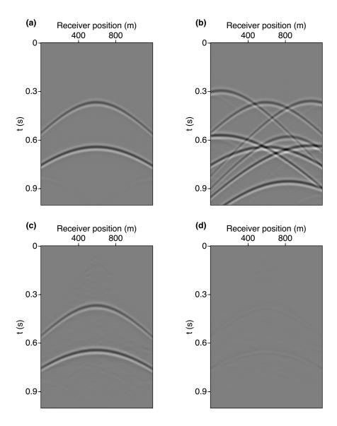
Figure 5.6: Results of deblending via the proposed algorithm for the two-layer model. (a) Ideal unblended shot gather (center shot) (b) Pseudo-deblended shot gather (c) Deblended shot gather after 30 iterations of gradient projection in the least-squares migration. The interferences are effectively suppressed.
