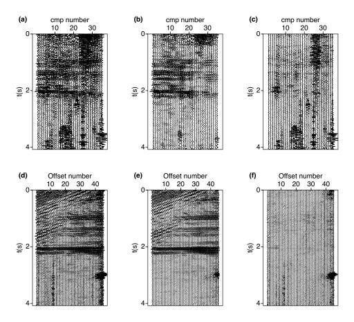
Figure C.2: RPCA de-noising for the Alaska data. (a) The original common offset gather before RPCA denoising. (b) Common offset gather after applying RPCA. (c) Difference bettween (a) and (b). (d) The original common midpoint gather before RPCA denoising. (e) Common midpoint gather after applying RPCA. (f) Difference between (d) and (e).
