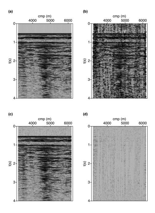
Figure 3.17: Results of simultaneous source separation of a 2D marine line: (a) The real unblended common offset gather. (b) (b) Common offset gather sorted from Pseudo-deblended data. (c) Deblended result via the proposed algorithm. (d) Differences between (a) and (c).
