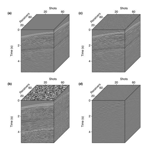
Figure 4.12: Results of deblending and reconstruction for whole data volume. (a) The original data from the Gulf of Mexico. (b) Pseudo-deblended data. (c) Deblended and reconstructed data after 30 iterations. (d) Difference section between original and deblended data.
