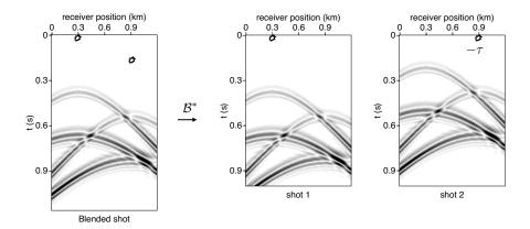
Figure 1.6: Illustration of pseudo-deblending of two shots. The time delay  $\tau$  is shifted back for shot 2. However, the interferences cannot be removed by pseudo-deblending.
