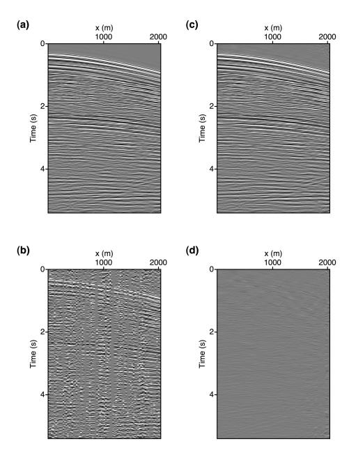
Figure 4.11: Results of deblending and reconstruction for a common receiver gather. (a) The original common receiver gather from a Gulf of Mexico dataset. (b) Pseudodeblended common receiver gather after numerical blending. (c) Deblended and reconstructed common receiver gather after 30 iterations. (d) Difference section between original and deblended data.
