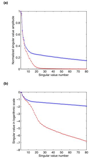
Figure 3.1: Distribution of singular values of spatial data in normal (a) and logarithmic (b) scale at 20Hz from the true unblended common receiver gather in f - x - y domain (red). We also portray the distribution of singular values for data contaminated with source interferences in a pseudo-deblended common receiver gather (blue).
