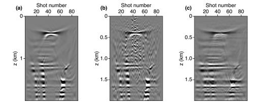
Figure 5.15: Migration results for Marmousi2 model: a shot-index common image gather (x=2km) (a) A shot-index common receiver gather from conventional unblended shot-profile migration; (b) A shot-index common receiver gather from blended shot-profile migration; (c) A shot-index common receiver gather from blended least-squares shot-profile migration.
