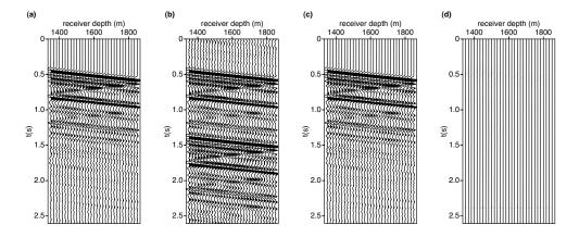
Figure 3.9: Results of simultaneous source separation in common shot domain when STR equals to 2: (a) The real unblended common shot gather (centre shot). (b) Pseudo-deblended shot record. (c) Deblended shot record after 20 iterations. (d) Differences between (a) and (c).In this example, the signal-to-noise ratio after separation is 36.5dB.
