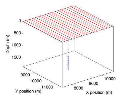
Figure 3.3: Distribution of sources and receivers of the 3D VSP data set. The sources are deployed on a regular grid in the surface and the receivers are deployed between 1350m and 1850m in the subsurface. Each red point represents a group of 10 sources and each blue triangle represents 5 receivers.
