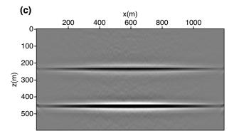
Figure 5.5: Migration results of the two-layer model: stacked image (a) Stacked image from conventional unblended shot-profile migration; (b) Stacked image from the blended shot-profile migration; (c) Stacked image from the blended least-squares shot-profile migration.
