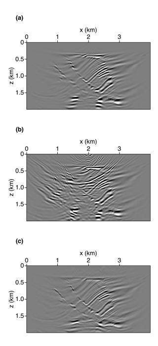
Figure 5.16: Migration results for Marmousi2 model: a partial image for a shot  $(S_x = 2.5km)$ . (a) A partial image from conventional unblended shot-profile migration; (b) A partial image from the blended shot-profile migration; (c) A partial image from the blended least-squares shot-profile migration.
