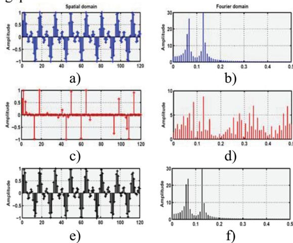
**Figure2:** a) Original signal; c) Signal with 80% randomly missing samples; e) Reconstructed signal using sparsity constraint. b, d, f) Fourier representations of a, c, e, respectively.
