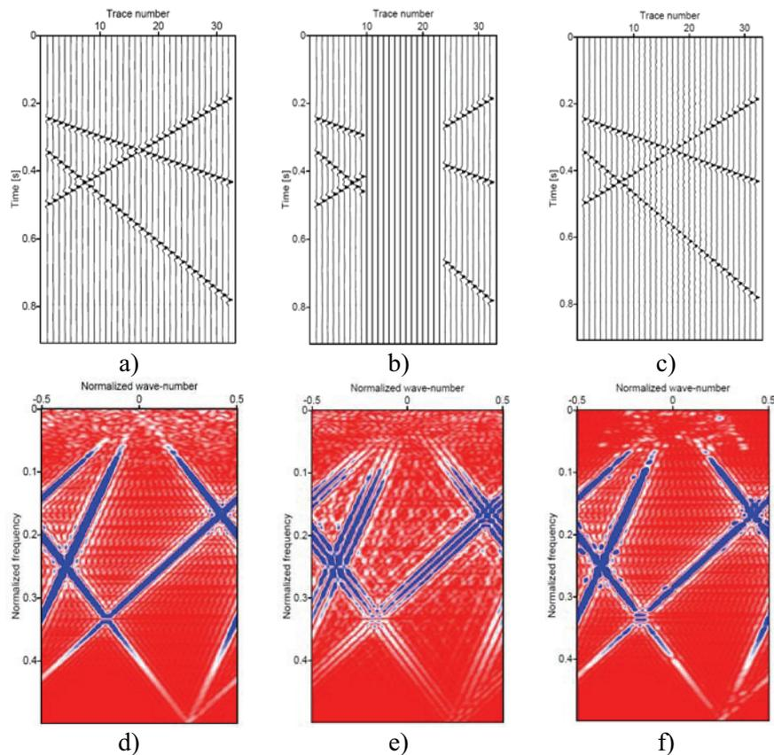
**Figure4:** a) Original 2D synthetic data; b) Data with gap; c) sparse reconstruction of b. d, e, f) Fourier representations of a, b, c, respectively.
