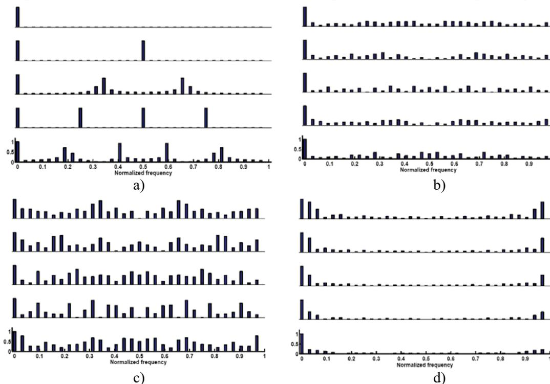
**Figure1:** Representations of scaling function for a) Regular decimation of signal; b,c) random sampling with 50% and 90% missing samples, respectively; d) gap inside the data
