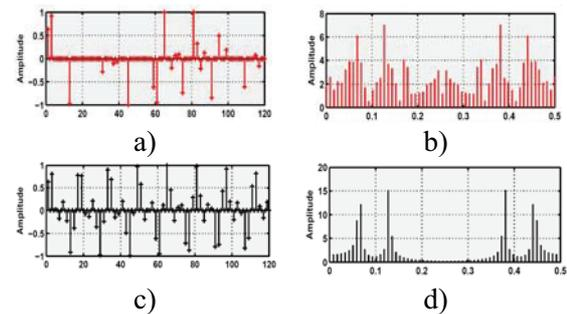
**Figure3:** a) Signal with 80% missing samples. Samples are picked from the decimated signal by factor of 2. c) Sparse reconstruction of a. b, d) Fourier representations of a, c, respectively.
