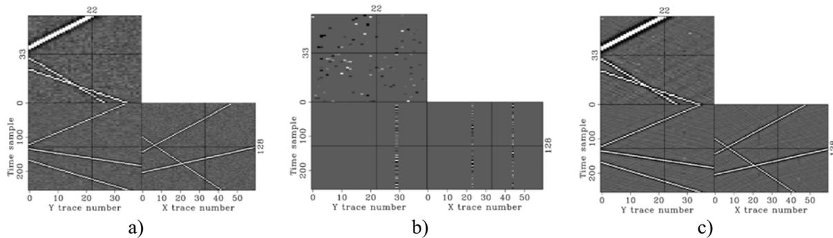
**Figure 5:** a) Original 3D synthetic data b) 90% randomly missing data c) sparse reconstruction result
