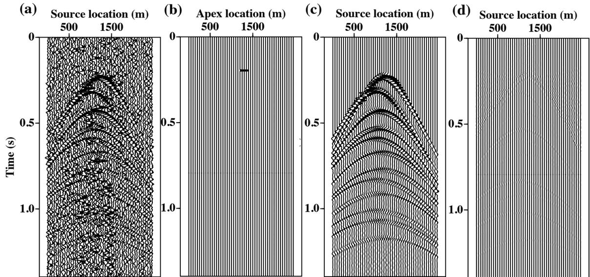
**Figure 3** Synthetic data common receiver gather. (a) Pseudodeblended gather. (a) Stolt model for one velocity estimated using  $p = 1, q = 1$  inversion. (c) Data recovered by forward modelling  $p = 1, q = 1$  estimated model. (d) Error in recovered data.
