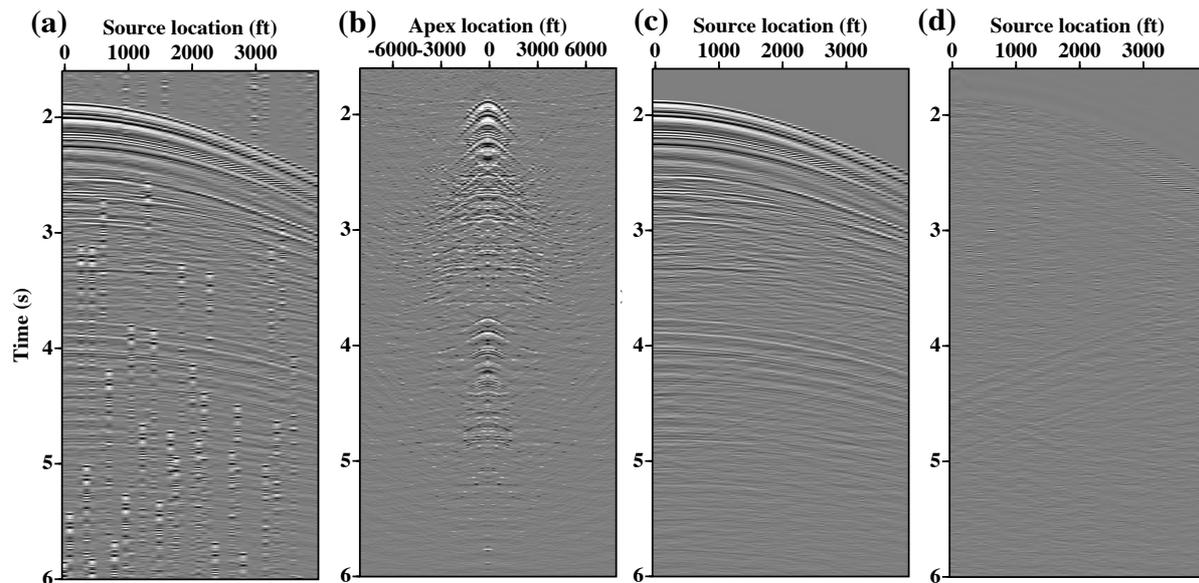
**Figure 4** Real data common receiver gather. (a) Pseudodeblended gather. (a) Stolt model for one velocity estimated using  $p = 1, q = 1$  inversion. (c) Data recovered by forward modelling  $p = 1, q = 1$  estimated model. (d) Error in recovered data.
