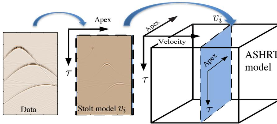
**Figure 1** Stolt operator used to compute ASHRT model.
