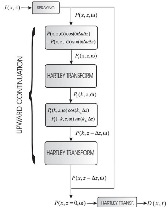
Fig. 2: The flowchart for split-step modeling using the Hartley transform. The wave field  $P(x, z, t = 0) = I(x, z)$  is propagated from the interior of the earth to the surface  $z = 0$  where the data  $D(x, t)$  is generated.
