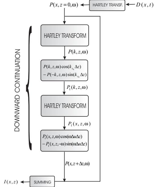
Fig. 1: The flowchart for the split-step migration using the Hartley transform. The wave field  $P(x, z = 0, t) = D(x, t)$  is propagated from the surface of the earth to depth  $z$  in steps  $\Delta z$ . The seismic image  $I(x, z)$  is constructed by applying the imaging principle .
