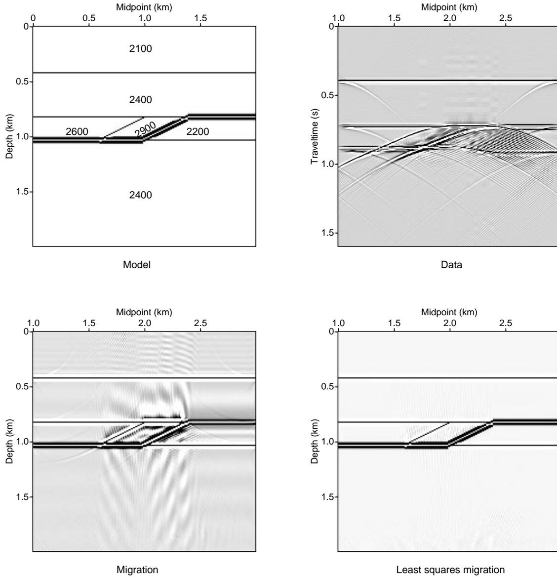
Fig. 3: A reflectivity model convolved with a Ricker wavelet is used to test the least-squares split-step migration. The interval velocities are given in meters per second. The data is generated using the forward split-step modeling operator. The split-step migrated section shows typical migration artifacts. In the least squares migrated image the artifacts are widely removed and the reflectivity is closer to that of the true model after only five iterations of the conjugate gradients scheme.
