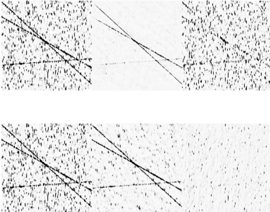
Fig. 2: Top: SNR enhancement using  $f-x$  prediction error filters assuming an AR model (Canales, 1984). Bottom: SNR enhancement using an ARMA model. In both figures we portray the noisy data (left), the filtered data (center), and the residual panel (right).
