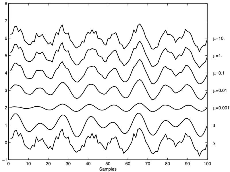
Fig. 1: The true signal  $s_k$  and the noisy signal  $y_k$  are displayed together with the estimated “clean signal” as a function of the tradeoff parameter  $\mu$  (equation (12)). The optimum tradeoff parameter  $\mu = 0.01$  yields a noise sequence with standard error  $\hat{\sigma} = 0.14$ . The standard error of the original noise sequence used to generate  $y_k$  is  $\sigma = 0.15$ .
