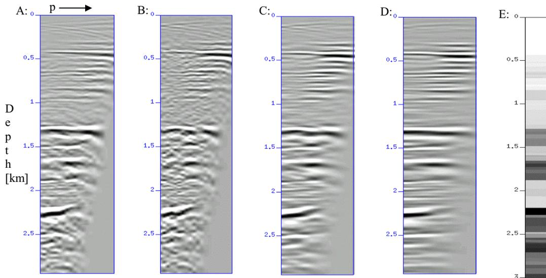
Figure 1: CAI gathers and velocity profile of CMP 175 of the Marmousi dataset. A: The CAI gather of the complete Marmousi dataset. B: CAI gather of the reduced dataset. About 80% of the shots have been randomly removed. C: The same CMP after 3 iterations of the CG algorithm with 1% smoothing. D: Result after 6 iterations using the same tradeoff parameter as in C. E: The velocity profile at CMP 175.
