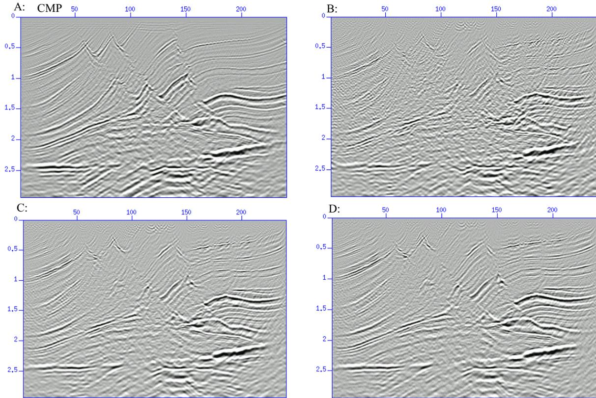
Figure 2: CAI images with a constant offset ray parameter of  $160 \mu\text{sec/m}$ . A: Constant offset ray parameter migration of the complete dataset. B: Constant offset ray parameter migration of the incomplete dataset (80% of the shots are set to zero). C: LS migration with ray parameter smoothing of the incomplete data after 3 iterations of the CG algorithm. D: Result after 6 iterations of the CG algorithm.
