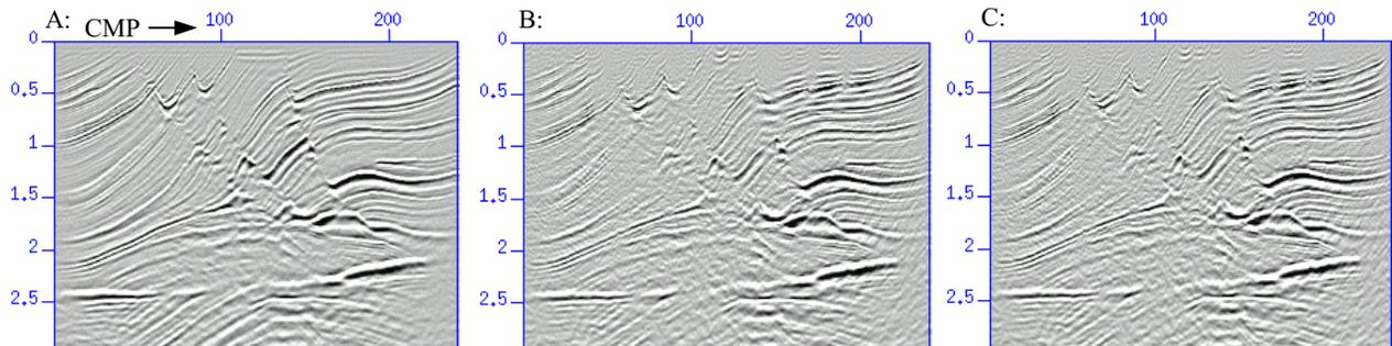
Figure 3: A: The stacked CAI gathers of the complete dataset. B and C show the stacked migration and the stacked LS migration (6 iterations with ray parameter smoothing) of the reduced dataset, respectively. Note the robustness of DSR migration with respect to missing data. The conventional migration and the LS migrated images (B and C) are almost identical. This can be explained by the tremendous healing effect of stacking.
