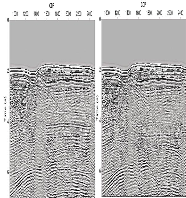
Figure 3. Left: Stacked section from the Gulf of Mexico. Right: Stacked section after fast HRT de-multiple.
