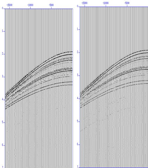
Figure 2. CMP gather after Hyperbolic Radon de-multiple. Left: least squares Hyperbolic Radon transform (HRT). Right: fast HRT.
