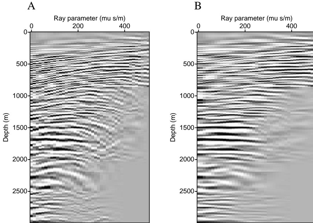
Fig. 2: (A) AVP gather obtained via direct migration of the pre-stack volume after binning. Null traces were assigned to missing offset positions. (B) AVP gather obtained via LS wave equation AVP migration after 4 conjugate gradients iterations.
