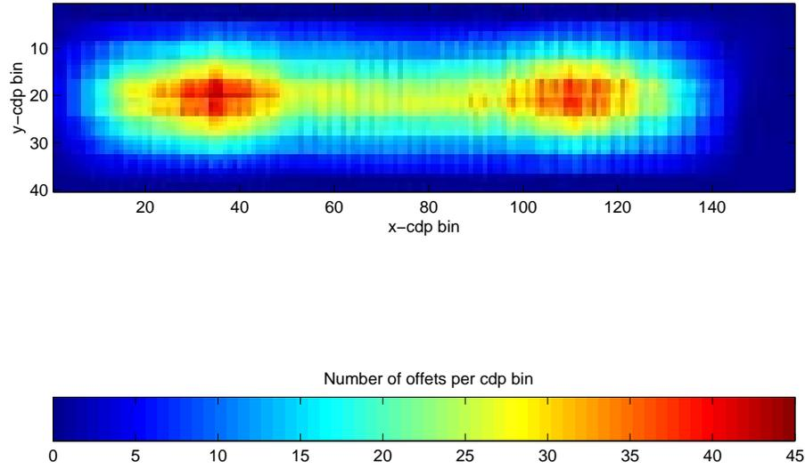
Fig. 1: Distribution of offset for the field data utilized to test our least-squares 3D wave equation AVA imaging algorithm.
