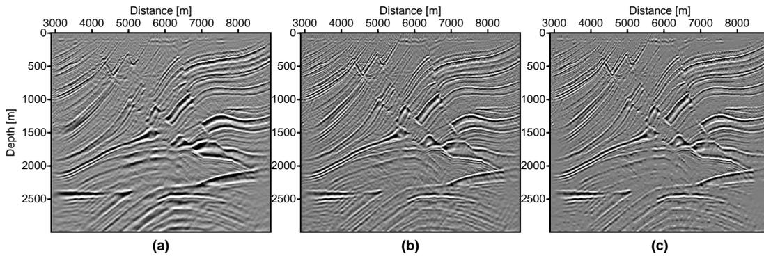
Fig. 3: Stacked images of the Marmousi data. (a) Migration. (b) PLSM. (c) SLSM.
