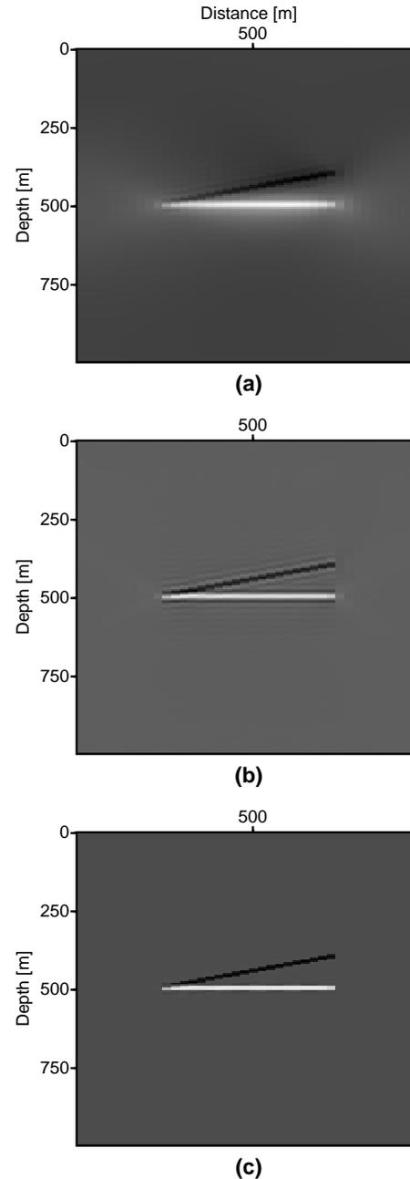
Fig. 1: Stacked images by migration, PLSM and SLSM. (a) Migration. (b) PLSM. (c) SLSM
