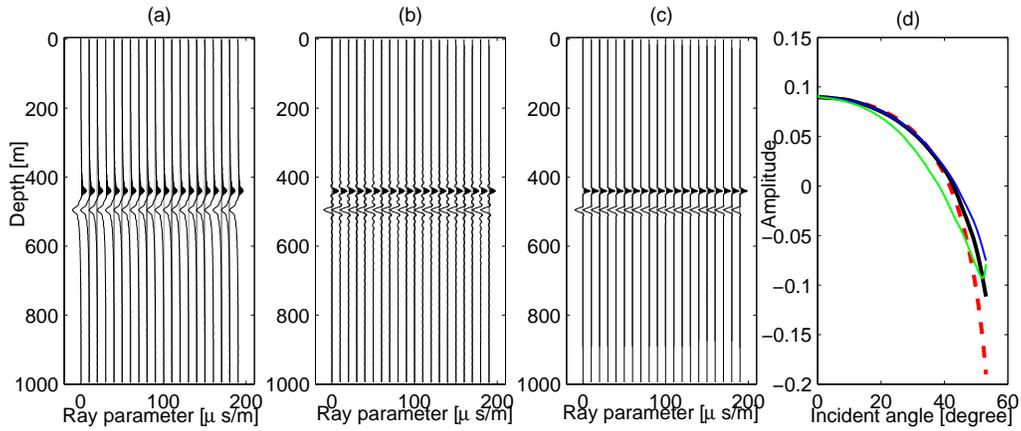
Fig. 2: Common image gathers (CIGs) and AVA curves at  $x = 500m$  for the wedge model. (a) Migration. (b) Preconditioned least-squares migration (PLSM). (c) Sparse least-squares migration (SLSM). (d) AVA curves for the first event. Red dashed: the theoretical curve. Green: migration. Blue: PLSM. Black: SLSM.
