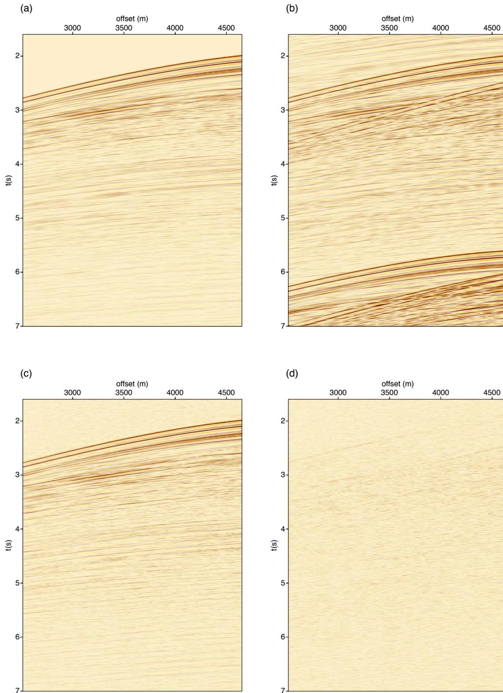
Figure 3: Results of separation via Iterative Rank Reduction method: (a) The real unblended shot record (20th). (b) Pseudo-deblended shot record. (c) Shot record separated with singular value projection. (d) Differences between (a) and (c)
