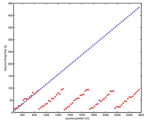
Figure 2: Temporal and spatial source distribution of simultaneous source separation. Each time 5 shots are recorded by a same set of receivers
