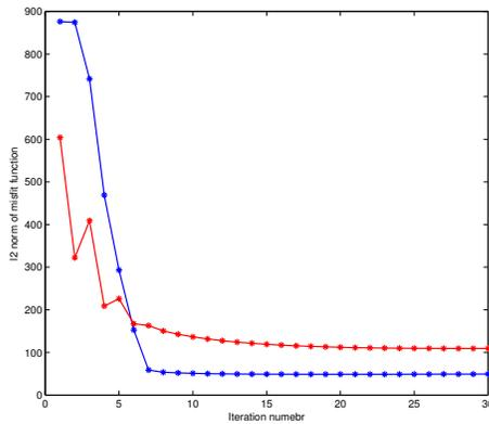
Figure 1: Convergence of iterative rank reduction source separation algorithm. Blue line indicates the  $l_2$  norm of the difference between the blended observations and the synthesized blended observation versus iteration. We also portray in blue the difference between the unblended data and the true data versus iteration.
