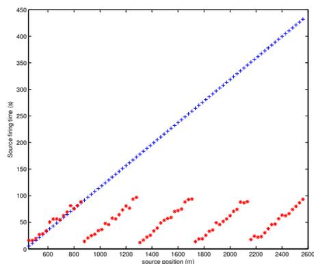
Figure 2: Temporal and spatial source distribution of simultaneous source separation. Each time 5 shots are recorded by a same set of receivers
