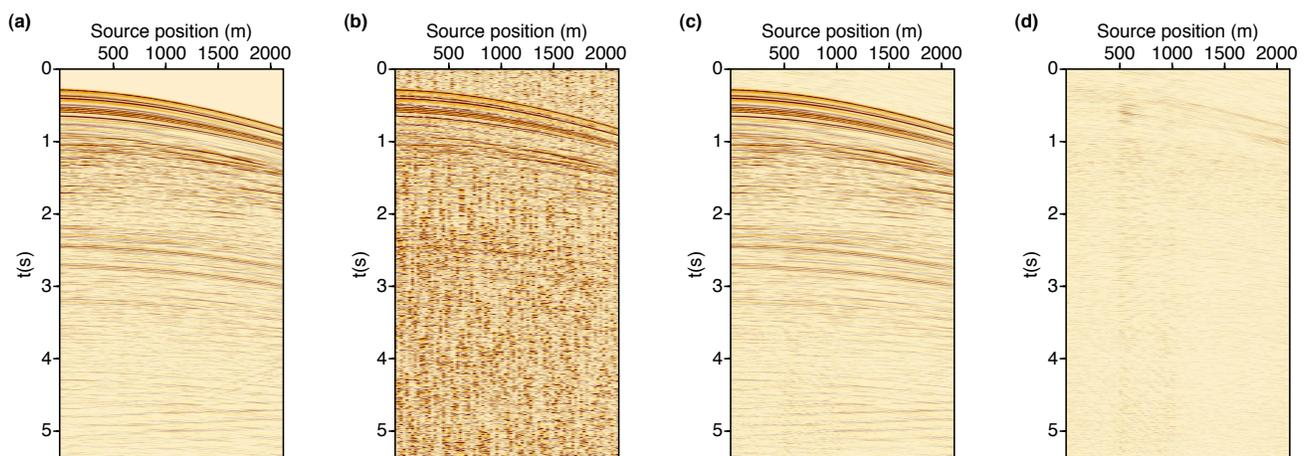
Figure 5: Results of source separation for the optimal firing scheme when STR equals to 3: (a) The real unblended common receiver gather. (b) Common receiver gather after pseudo-deblending. (c) Common receiver gather after source separation and reconstruction. (d) Differences between (a) and (c).
