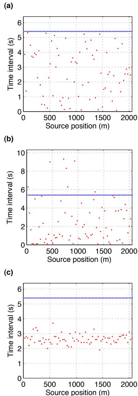
Figure 1: Distribution of time delays versus source position: (a) Uniform distribution. (b) Exponential distribution. (c) Binomial distribution. In this example, the STR equals to 2.
