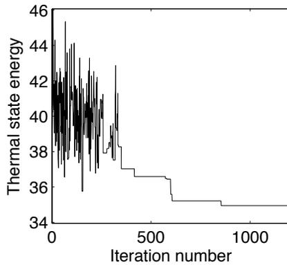
Figure 3: Thermal state energy versus iteration numbers in fast simulated annealing.
