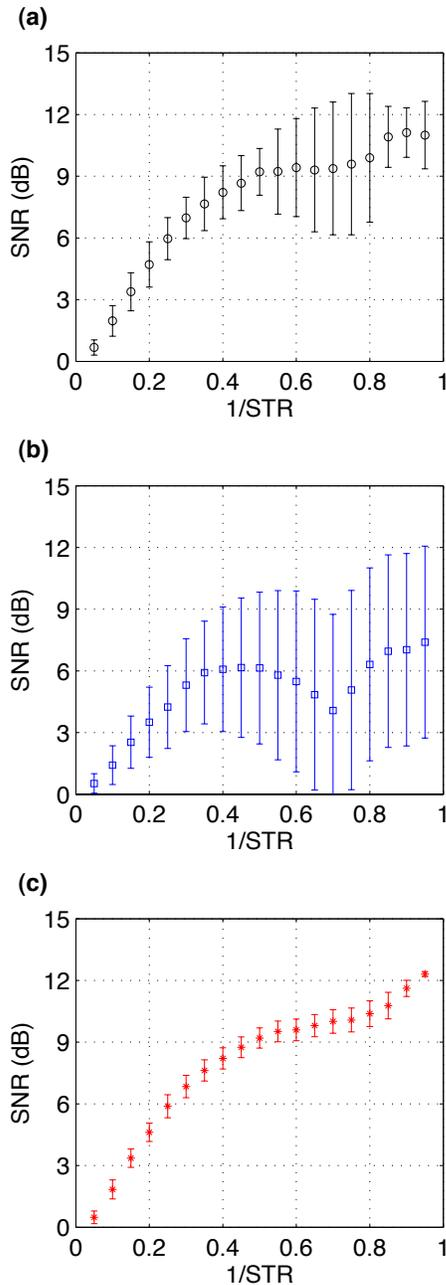
Figure 2: SNR of the deblended common receiver gather versus the inverse of STR: (a) Uniform distribution. (b) Exponential distribution. (c) Binomial distribution. Binomial distributions shows the most stable performance for deblending.
