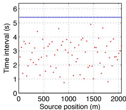
Figure 4: Optimal time delays inverted via fast simulated annealing. In this example, the STR equals to 2.
