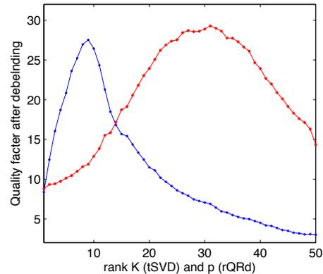
Figure 2: The quality of debblending versus rank  $K$  in tSVD and  $p$  for the rQRd. The blue curve shows the results utilizing the truncated SVD as the low rank projection operator while the red is the results corresponding to the rQRd method.
