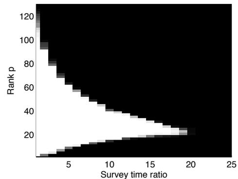
Figure 3: The probability map of simultaneous source separation with the proposed debblending method under different rank and survey time ratio. For small STRs, a broad range of ranks could be adopted to achieve successful separations. As the STR grows, we need precise knowledge of the optimum rank to correctly debblend the data. For this specific model and acquisition design, the algorithm performs poorly when STR is greater than 21.
