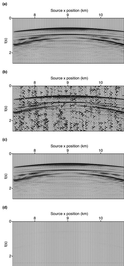
Figure 5: Results of simultaneous source separation in common receiver domain: (a) The real unblended common receiver gather. (b) Pseudo-deblended common receiver gather. (c) Deblended common receiver gather via the proposed algorithm. (d) Differences between (a) and (c).
