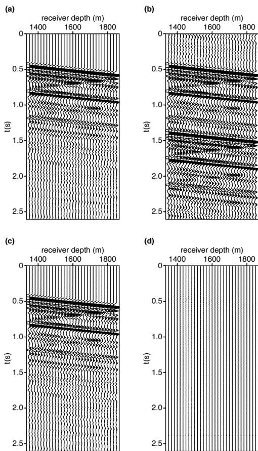
Figure 4: Results of simultaneous source separation in common shot domain. STR equals to 2. (a) The real unblended common shot gather. (b) Pseudo-deblended common shot gather. (c) Deblended common shot gather via the proposed algorithm. (d) Differences between (a) and (c). In this example, the signal-to-noise ratio after separation is 32.5dB.
