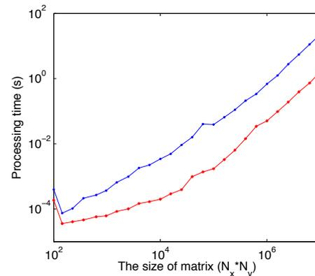
Figure 1: Processing time of rank reduction versus size of the matrix in logarithmic scale. The blue curve shows the processing time for the truncated SVD. The red curve corresponds to the rQRd method. In this example, we choose  $p$  equals to 3K
