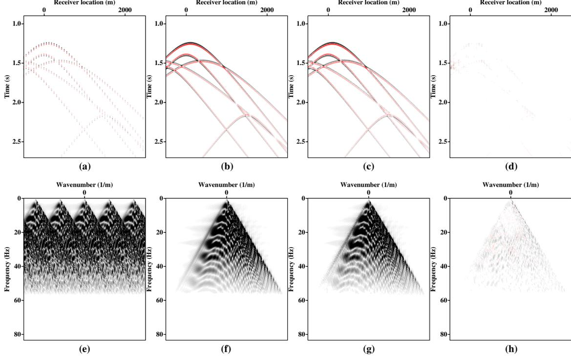
Figure 1: Simplified synthetic shot gather example. (a) Decimated gather. (b) Original gather. (c) Interpolated gather. (d) Interpolation error. (e), (f), (g) and (h) are the  $\omega - k_x$  spectra of (a), (b), (c), and (d), respectively.
