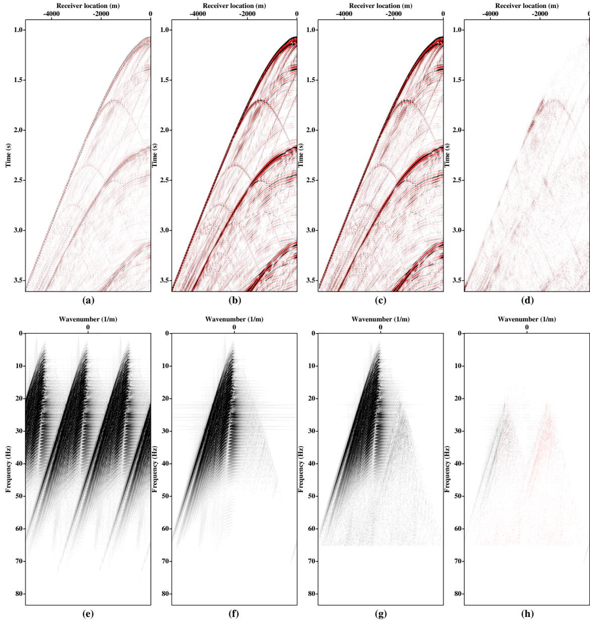
Figure 2: Shot gather example of the BP/SEG velocity model. (a) Decimated gather. (b) Original gather. (c) Interpolated gather. (d) Interpolation error. (e), (f), (g) and (h) are the  $\omega - k_x$  spectra of (a), (b), (c), and (d), respectively.
