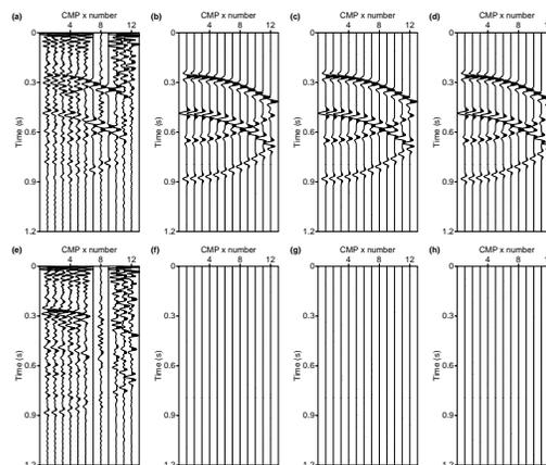
Figure 2: Slice view of reconstructed data for the noise-free data. a) TMF method. b) SMF method. c) PSMF method. d) PMF method. e), f), g) and h) are the difference of the subtraction of the true complete data and reconstructed data results.
