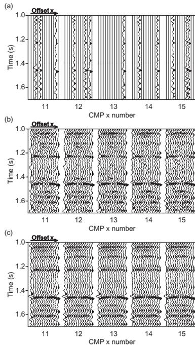
Figure 5: A CMPx gather reconstruction result of a real data for fixed CMPy bin=7, hy bin=7 and  $\mu=0.9$ . a) Input gathers. b) Reconstructed gathers using the PMF method. c) Reconstructed gathers using the PSMF method.
