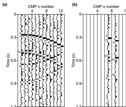
Figure 3: Slice view of noisy complete data with  $S/N=1.0$  a) and decimated data with 80% missing traces b).
