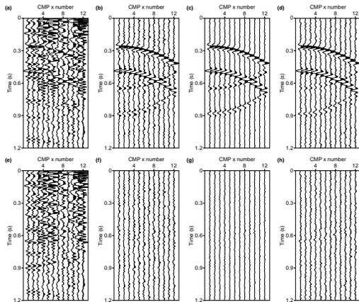
Figure 4: Slice view of reconstruction results for the noisy data set with 80% missing traces and  $\mu=0.1$ . a) TMF method. b) SMF method. c) PSMF method. d) PMF method. e), f), g) and h) are the difference of the subtraction of the true complete data and reconstructed data.
