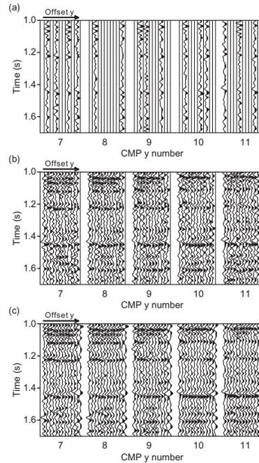
Figure 6: A CMPy gather reconstruction result of a real data for fixed CMPx bin=6, hx bin=6. a) Input gathers. b) Reconstructed gathers using the PMF method. c) Reconstructed gathers using the PSMF method.
