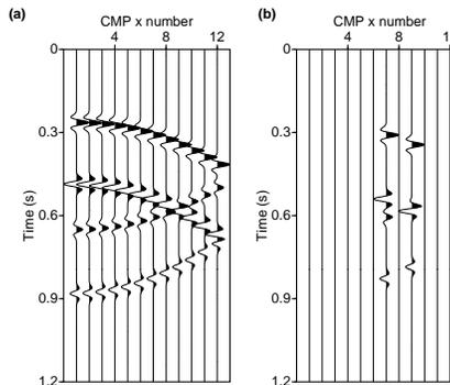
Figure 1: Slice view of original noise-free complete data a) and decimated data with 80% missing traces b).
