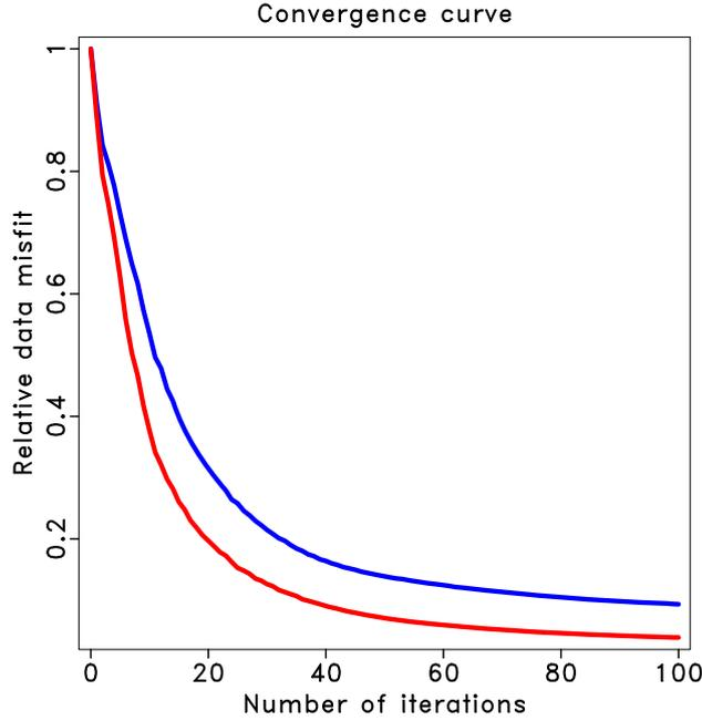
**Figure 5.** Comparison of the convergence curves of three-parameter elastic LSRTM (red) and two-parameter elastic LSRTM (blue) for elastic inclusion model.
