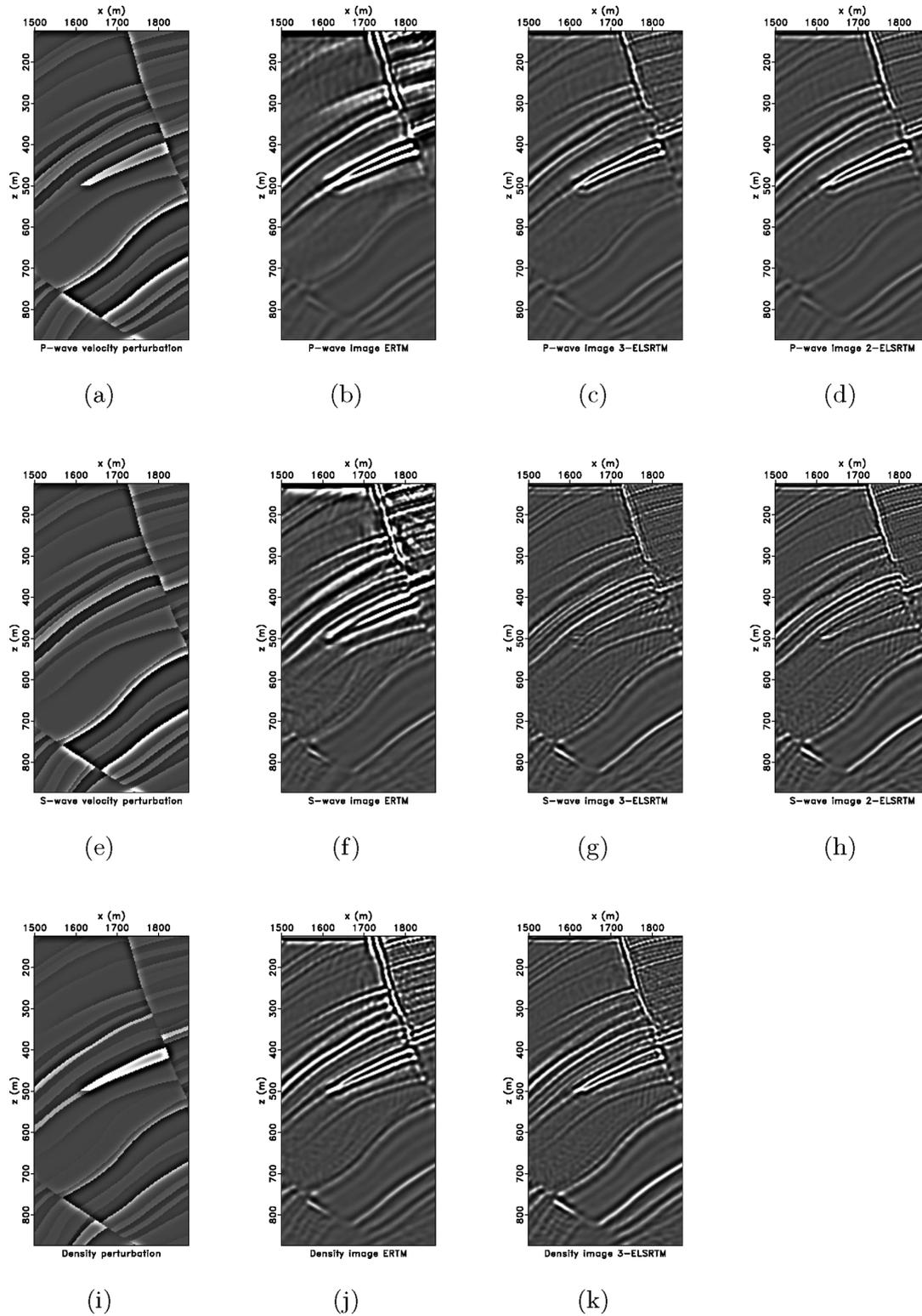
**Figure 11.** Comparison of images in the range  $1500 \text{ m} < x < 1875 \text{ m}$  and  $125 \text{ m} < z < 875 \text{ m}$ . *P*-wave velocity perturbation: (a) true model, (b) elastic RTM, (c) three-parameter elastic LSRTM, (d) two-parameter elastic LSRTM. *S*-wave velocity perturbation: (e) true model, (f) elastic RTM, (g) three-parameter elastic LSRTM, (h) two-parameter elastic LSRTM. Density perturbation: (i) true model, (j) elastic RTM, (k) three-parameter elastic LSRTM.
