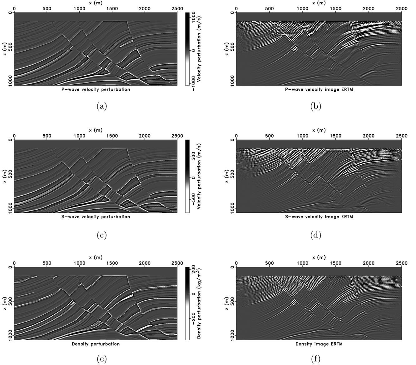
**Figure 8.** (a) True  $P$ -wave velocity perturbation. (b)  $P$ -wave velocity perturbation image estimated via elastic RTM. (c) True  $S$ -wave velocity perturbation. (d)  $S$ -wave velocity perturbation image estimated via elastic RTM. (e) True density perturbation. (f) Density perturbation image estimated via elastic RTM.
