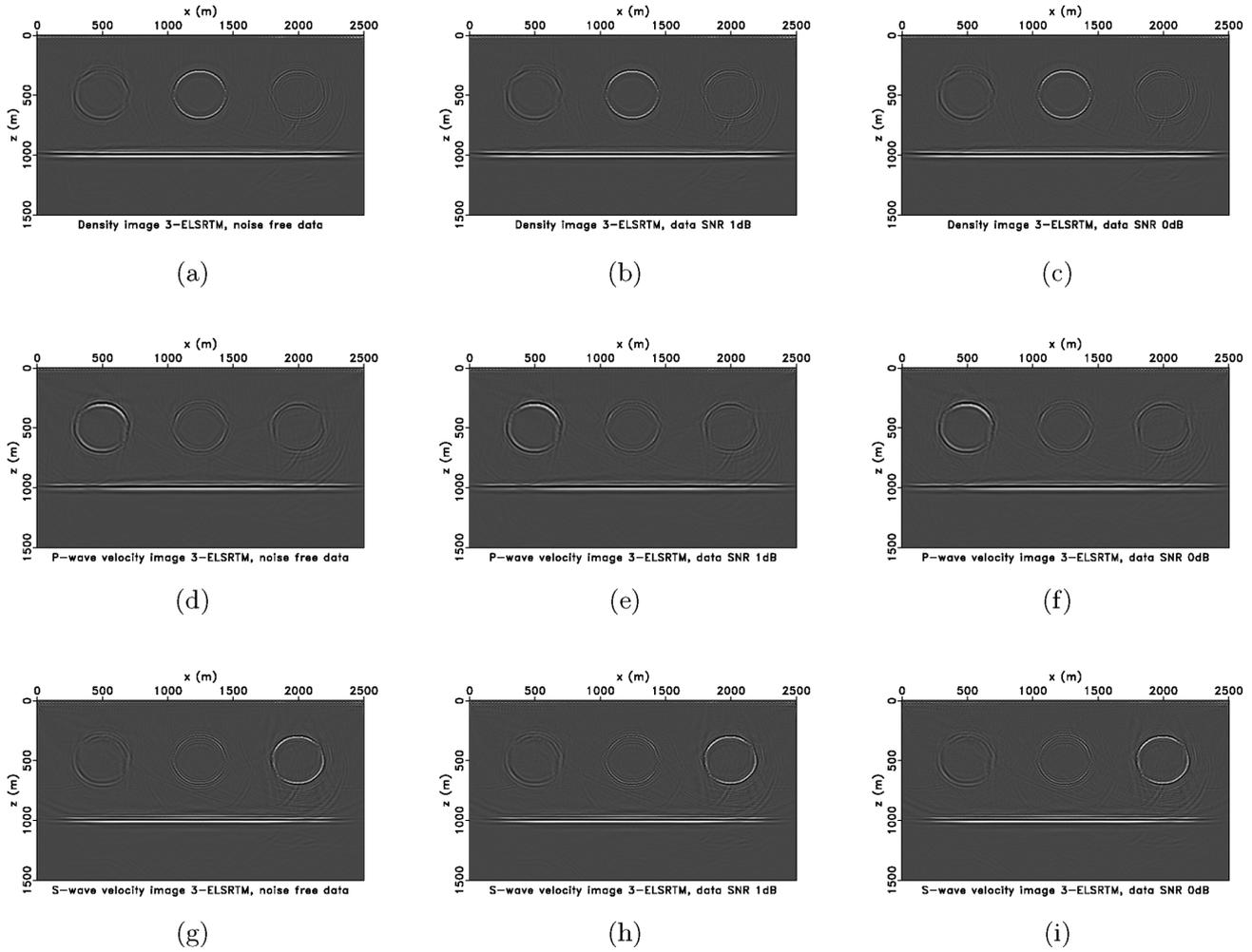
**Figure 15.** Three-parameter elastic LSRTM images using data with different SNRs. Estimated density images from noise-free data (a), data with SNR 1 dB (b) and data with SNR 0 dB (c). Estimated  $P$ -wave velocity images from noise-free data (d), data with SNR 1 dB (e) and data with SNR 0 dB (f). Estimated  $S$ -wave velocity images from noise-free data (g), data with SNR 1 dB (h) and data with SNR 0 dB (i).
