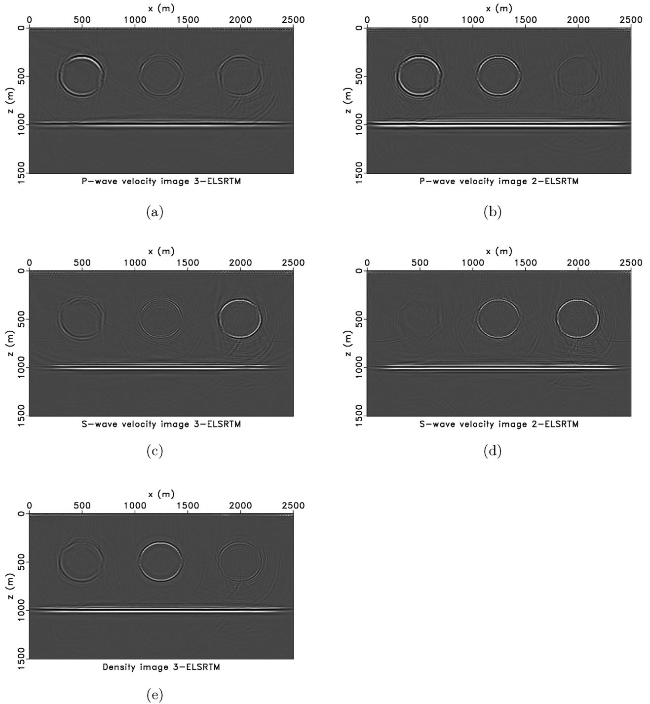
**Figure 4.**  $P$ -wave velocity perturbation image estimated via three-parameter elastic LSRTM (a) and two-parameter elastic LSRTM (b).  $S$ -wave velocity perturbation image estimated via three-parameter elastic LSRTM (c) and two-parameter elastic LSRTM (d). Density perturbation image estimated via three-parameter elastic LSRTM (e).
