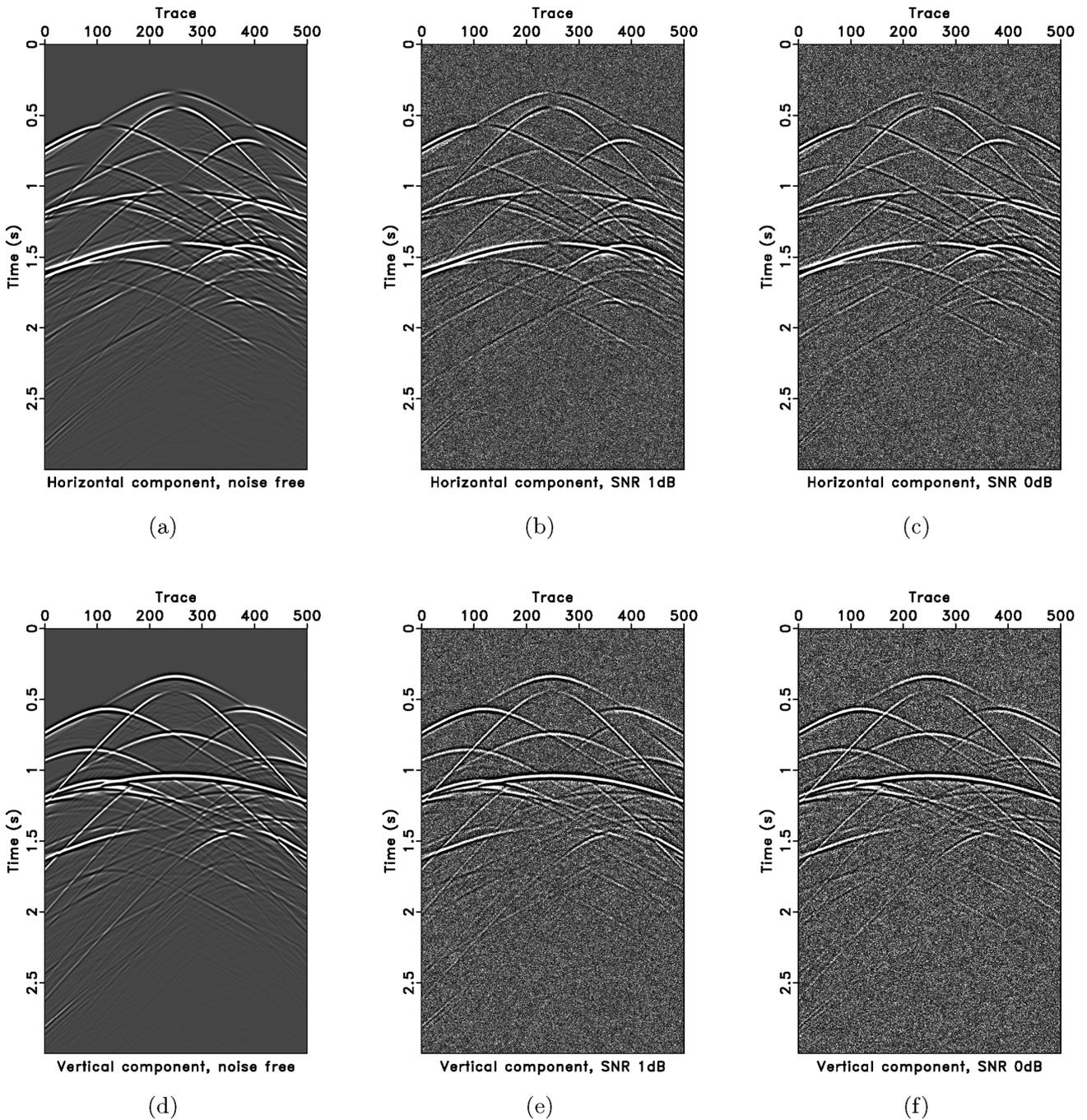
**Figure 14.** The 50th shot gather with different SNRs. (a) Noise-free horizontal component data. (b) Horizontal component data with SNR 1 dB. (c) Horizontal component data with SNR 0 dB. (d) Noise-free vertical component data. (e) Vertical component data with SNR 1 dB. (f) Vertical component data with SNR 0 dB.
