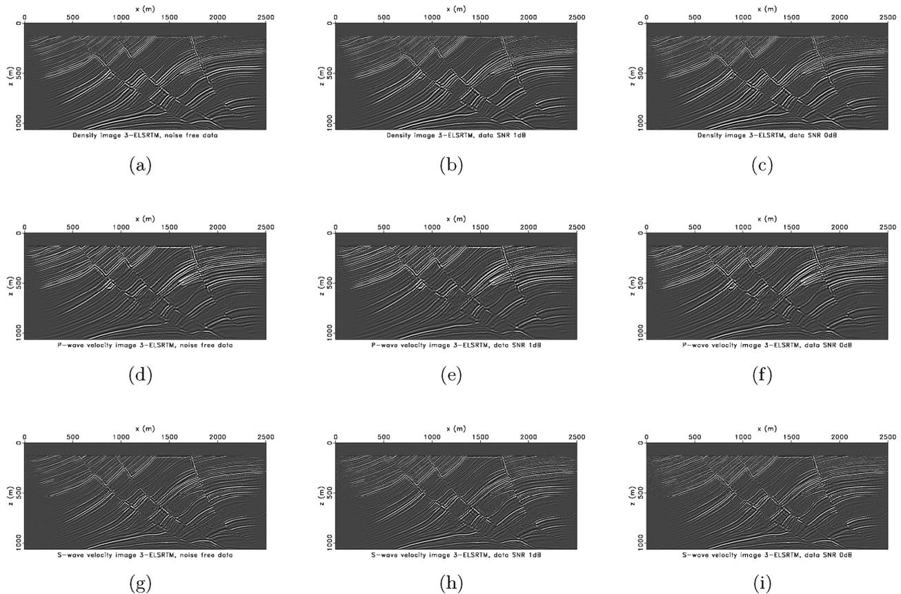
**Figure 17.** Three-parameter elastic LSRTM images using data with different SNRs. Estimated density images from noise-free data (a), data with SNR 1 dB (b) and data with SNR 0 dB (c). Estimated  $P$ -wave velocity images from noise-free data (d), data with SNR 1 dB (e) and data with SNR 0 dB (f). Estimated  $S$ -wave velocity images from noise-free data (g), data with SNR 1 dB (h) and data with SNR 0 dB (i).
