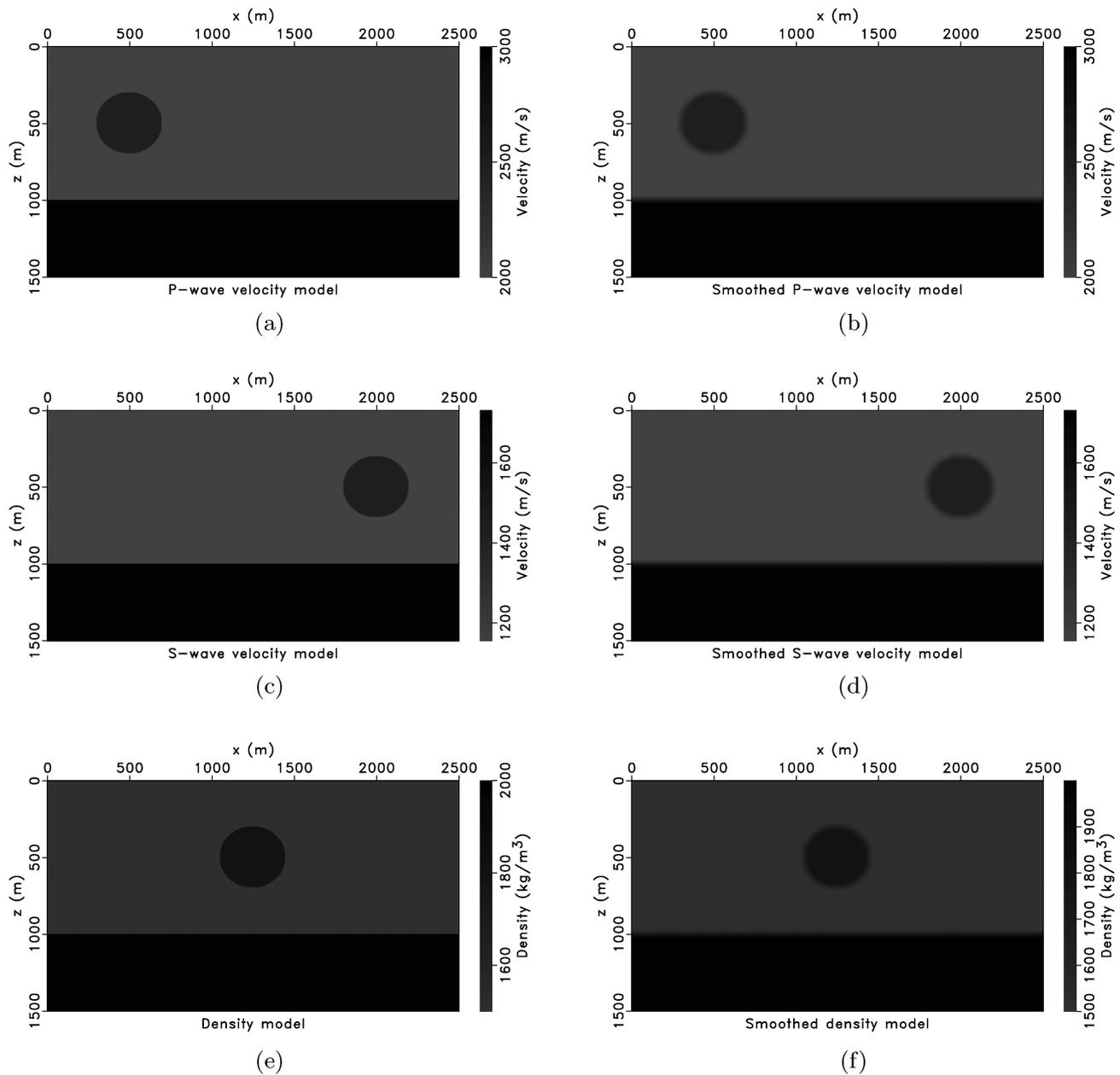
**Figure 1.** Elastic inclusion model. (a)  $P$ -wave velocity model. (b) Smoothed  $P$ -wave velocity model. (c)  $S$ -wave velocity model. (d) Smoothed  $S$ -wave velocity model. (e) Density model. (f) Smoothed density model.
