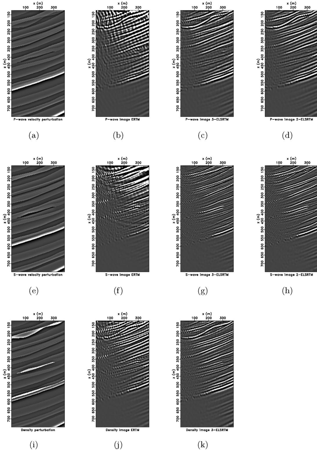
**Figure 12.** Comparison of images in the range  $0 \text{ m} < x < 375 \text{ m}$  and  $125 \text{ m} < z < 750 \text{ m}$ . *P*-wave velocity perturbation: (a) true model, (b) elastic RTM, (c) three-parameter elastic LSRTM, (d) two-parameter elastic LSRTM. *S*-wave velocity perturbation: (e) true model, (f) elastic RTM, (g) three-parameter elastic LSRTM, (h) two-parameter elastic LSRTM. Density perturbation: (i) true model, (j) elastic RTM, (k) three-parameter elastic LSRTM.
