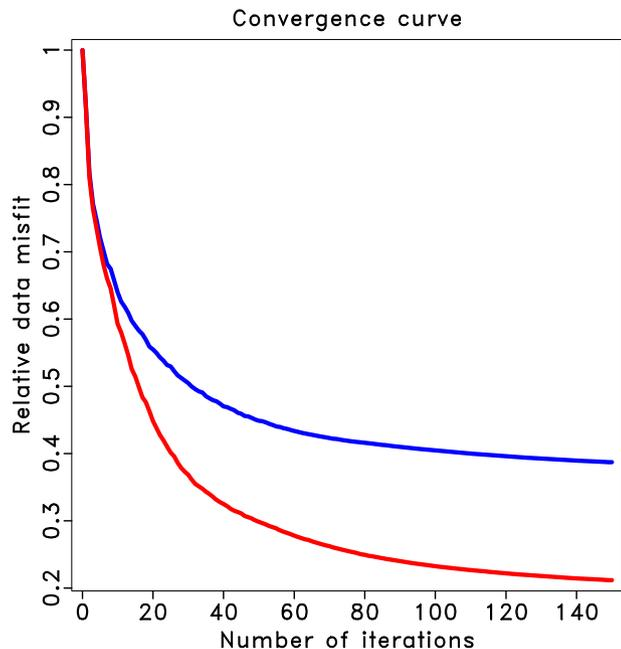
**Figure 13.** Comparison of the convergence curves of three-parameter elastic LSRTM (red) and two-parameter elastic LSRTM (blue) for elastic Marmousi2 model.
