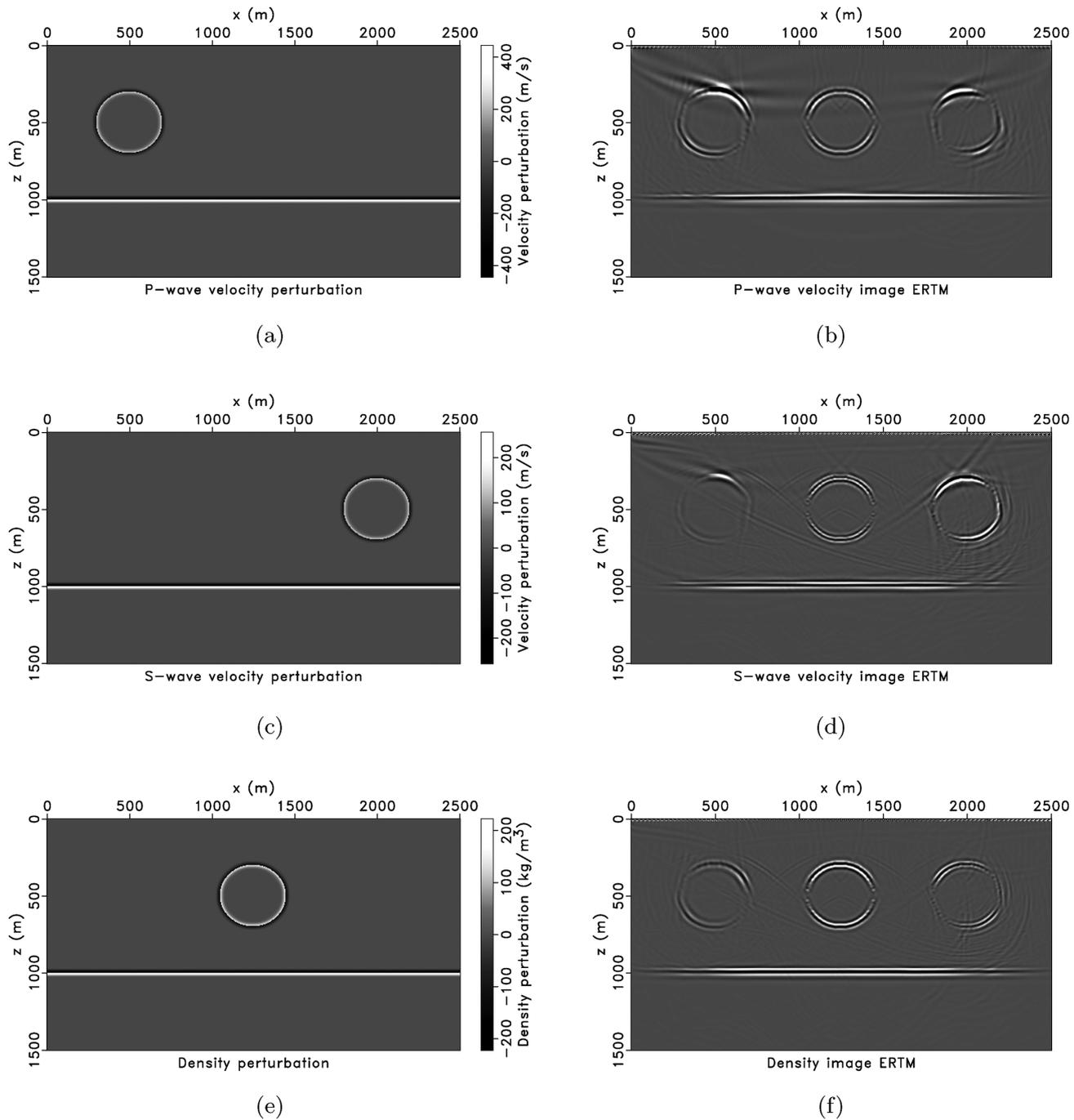
**Figure 3.** (a) True  $P$ -wave velocity perturbation. (b)  $P$ -wave velocity perturbation image estimated via elastic RTM. (c) True  $S$ -wave velocity perturbation. (d)  $S$ -wave velocity perturbation image estimated via elastic RTM. (e) True density perturbation. (f) Density perturbation image estimated via elastic RTM.
