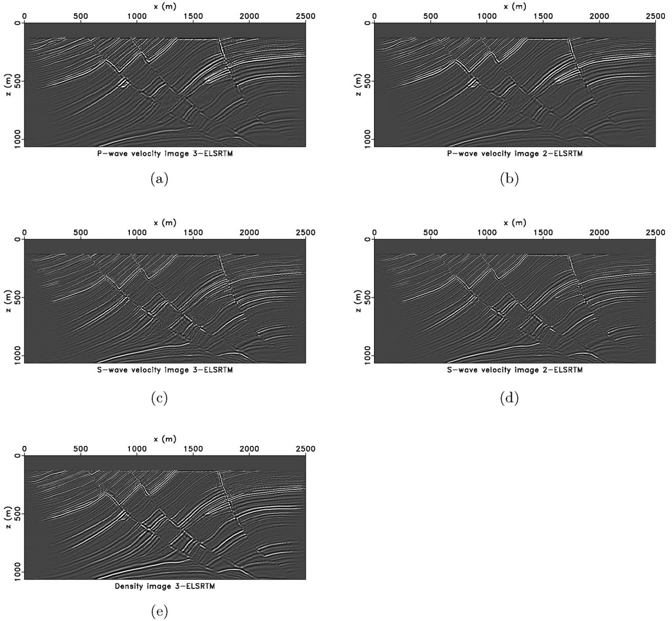
**Figure 9.** *P*-wave velocity perturbation image estimated via three-parameter elastic LSRTM (a) and two-parameter elastic LSRTM (b). *S*-wave velocity perturbation image estimated via three-parameter elastic LSRTM (c) and two-parameter elastic LSRTM (d). Density perturbation image estimated via three-parameter elastic LSRTM (e).
