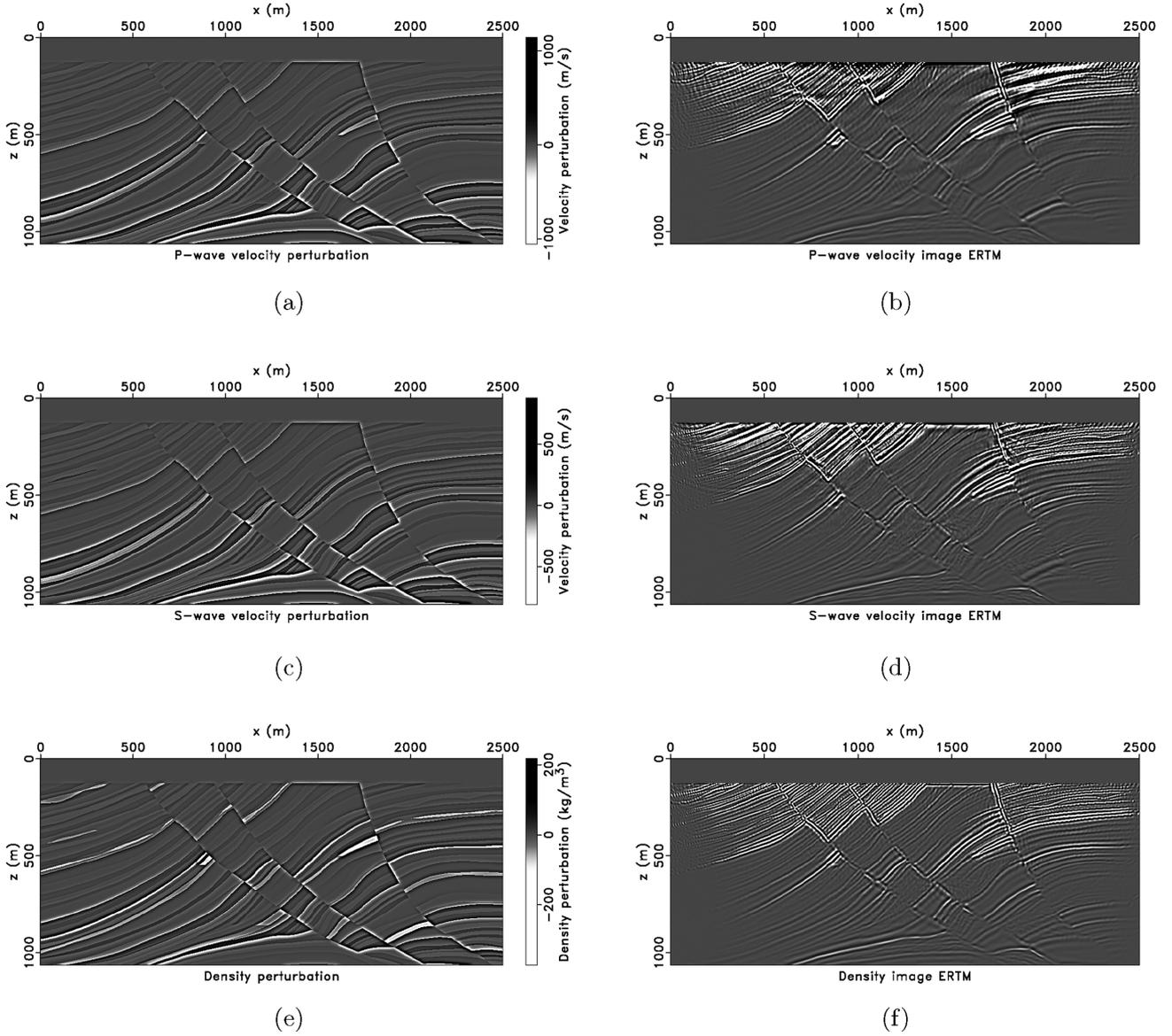
**Figure 8.** (a) True  $P$ -wave velocity perturbation. (b)  $P$ -wave velocity perturbation image estimated via elastic RTM. (c) True  $S$ -wave velocity perturbation. (d)  $S$ -wave velocity perturbation image estimated via elastic RTM. (e) True density perturbation. (f) Density perturbation image estimated via elastic RTM.
