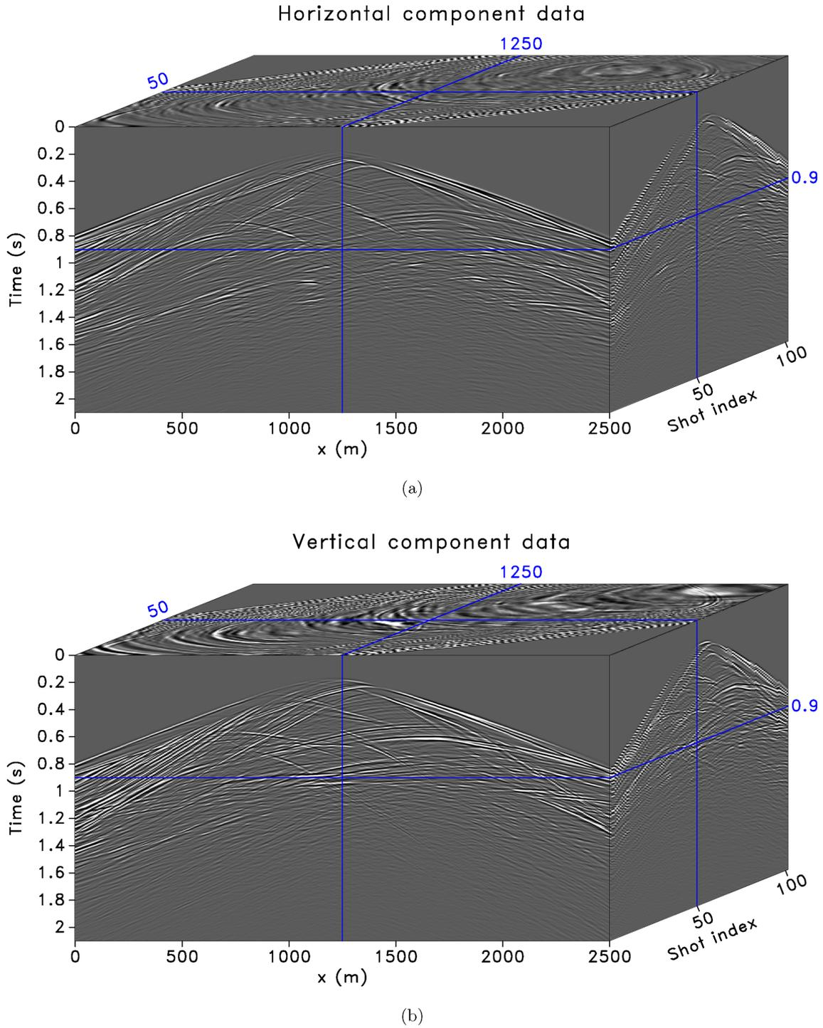
**Figure 7.** Multicomponent data of the elastic Marmousi2 model. (a) Horizontal particle velocity data. (b) Vertical particle velocity data.
