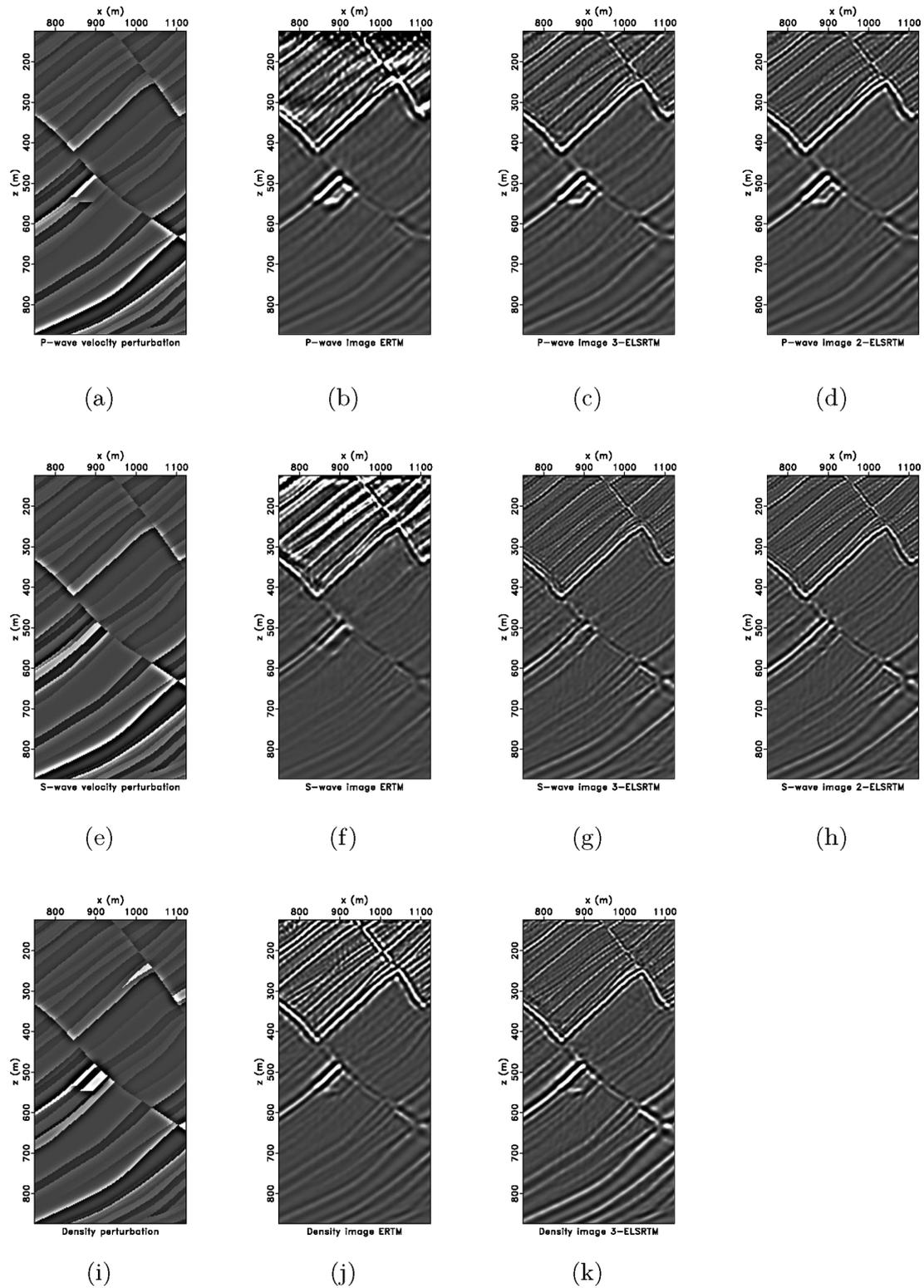
**Figure 10.** Comparison of images in the range  $750 \text{ m} < x < 1125 \text{ m}$  and  $125 \text{ m} < z < 875 \text{ m}$ . *P*-wave velocity perturbation: (a) true model, (b) elastic RTM, (c) three-parameter elastic LSRTM, (d) two-parameter elastic LSRTM. *S*-wave velocity perturbation: (e) true model, (f) elastic RTM, (g) three-parameter elastic LSRTM, (h) two-parameter elastic LSRTM. Density perturbation: (i) true model, (j) elastic RTM, (k) three-parameter elastic LSRTM.
