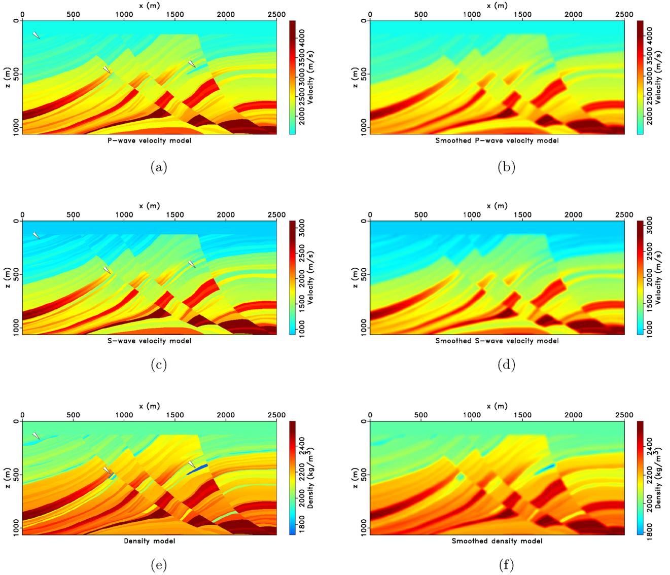
**Figure 6.** Elastic Marmousi2 model. (a)  $P$ -wave velocity model. (b) Smoothed  $P$ -wave velocity model. (c)  $S$ -wave velocity model. (d) Smoothed  $S$ -wave velocity model. (e) Density model. (f) Smoothed density model.
