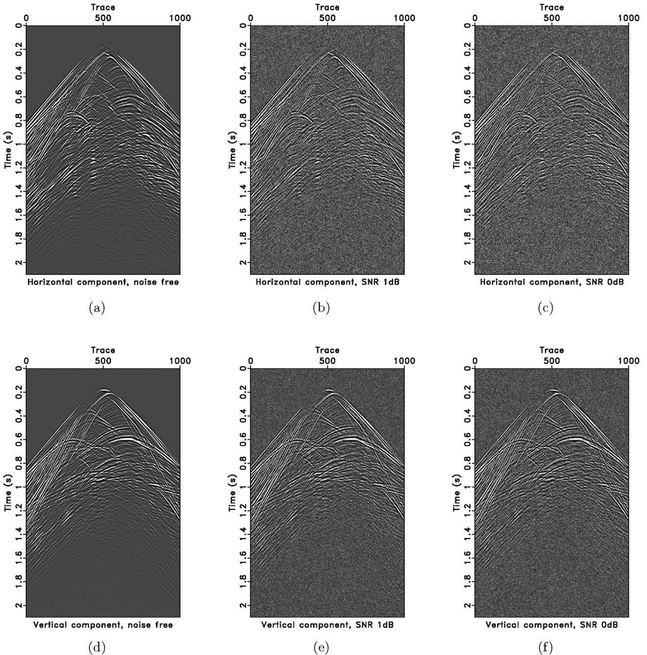
**Figure 16.** The 50th shot gather with different SNRs. (a) Noise-free horizontal component data. (b) Horizontal component data with SNR 1 dB. (c) Horizontal component data with SNR 0 dB. (d) Noise-free vertical component data. (e) Vertical component data with SNR 1 dB. (f) Vertical component data with SNR 0 dB.
