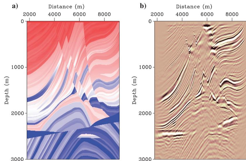
Figure 4. Velocity field of the Marmousi model and the corresponding shot-profile wave-equation-migrated image. (a) True velocity field. (b) Adjoint migrated model.
