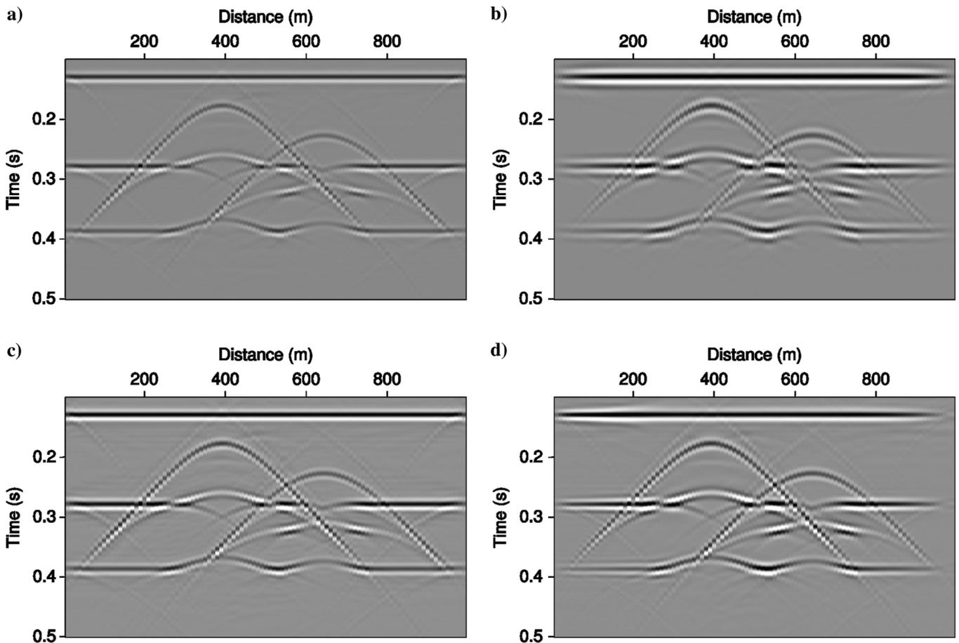
Figure 3. True and predicted near-offset sections. (a) True near-offset section. (b) Adjoint predicted section. (c) Least-squares predicted section. (d) Block row recursive least-squares predicted section.
