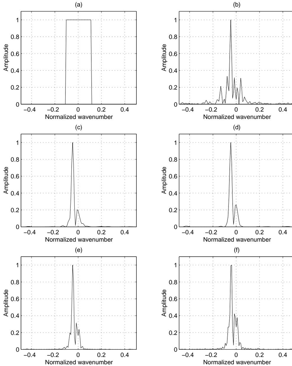
Figure 3.7: Analysis of the spectral weights  $P_k^2$  at frequency component  $f = 23$  Hz. (a) Unitary spectral weights used by the MNI method. (b) Power spectrum of the incomplete data, missing samples were filled in with zeros. (c) Spectral weights at the second iteration of the MWNI method. (d) The weighting function at the last iteration of the MWNI method. (e) The spectrum of reconstructed data using MWNI. (f) The spectrum of the original (complete) data.
