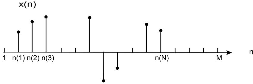
Figure 3.1: The band limited interpolation/extrapolation problem: the given time samples are  $x_{n(1)}, x_{n(2)}, x_{n(3)}, \dots, x_{n(N)}$  and are located in the interval  $[1, M]$ . The remaining samples in this interval are to be estimated.
