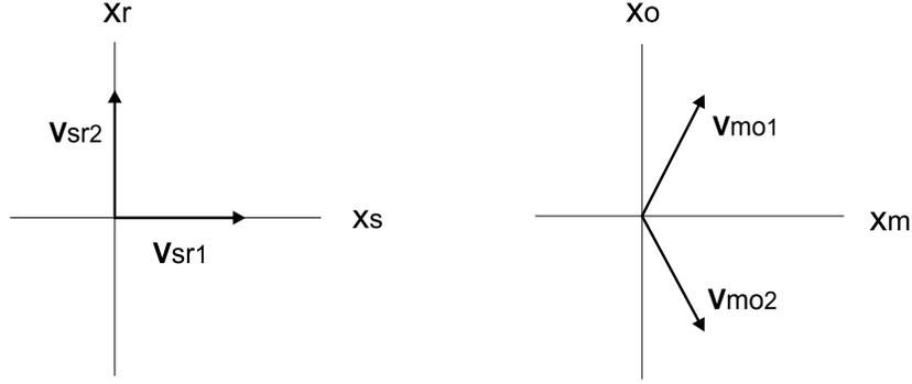
Figure 2.9: The sampling matrices in the shot-receiver domain and midpoint-offset domain. The shot-receiver domain sampling matrix is  $\underline{\mathbf{V}}_{sr} = [\mathbf{v}_{sr1} \ \mathbf{v}_{sr2}]$  and the midpoint-offset domain sampling matrix is  $\underline{\mathbf{V}}_{mo} = [\mathbf{v}_{mo1} \ \mathbf{v}_{mo2}]$ .
