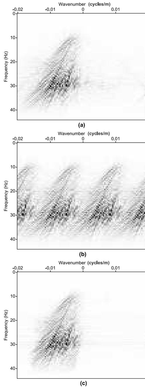
Figure 3.17: (a) The  $f-k$  spectrum of the original shot gather at 3125 m. (b) The  $f-k$  spectrum of the same shot gather after decimation (Notes the decimated shot data has been filled with zero traces in the missing trace positions). (c) The  $f-k$  spectrum of the same shot gather after interpolation.
