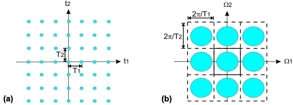
Figure 2.5: Periodic sampling of a 2-D continuous signal with rectangular geometry. (a) Sampling locations on the 2-D plane. (b) Replication of the original spectrum after periodic sampling.
