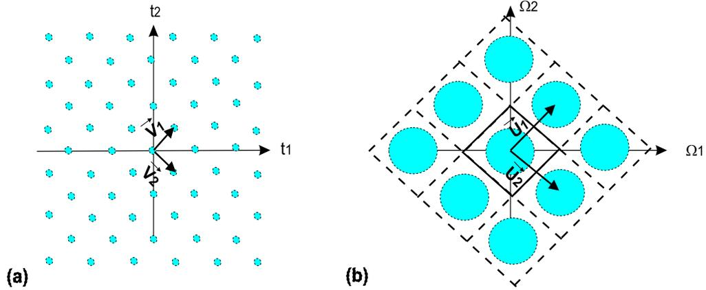
Figure 2.6: Periodic sampling of a 2-D continuous signal with arbitrary geometry. (a) Sampling locations in the  $(t_1, t_2)$ -plane determined by the vectors  $\mathbf{v}_1$  and  $\mathbf{v}_2$  which comprise the sampling matrix  $\mathbf{V}$ . (b) Replications of the original spectrum after the periodic sampling.
