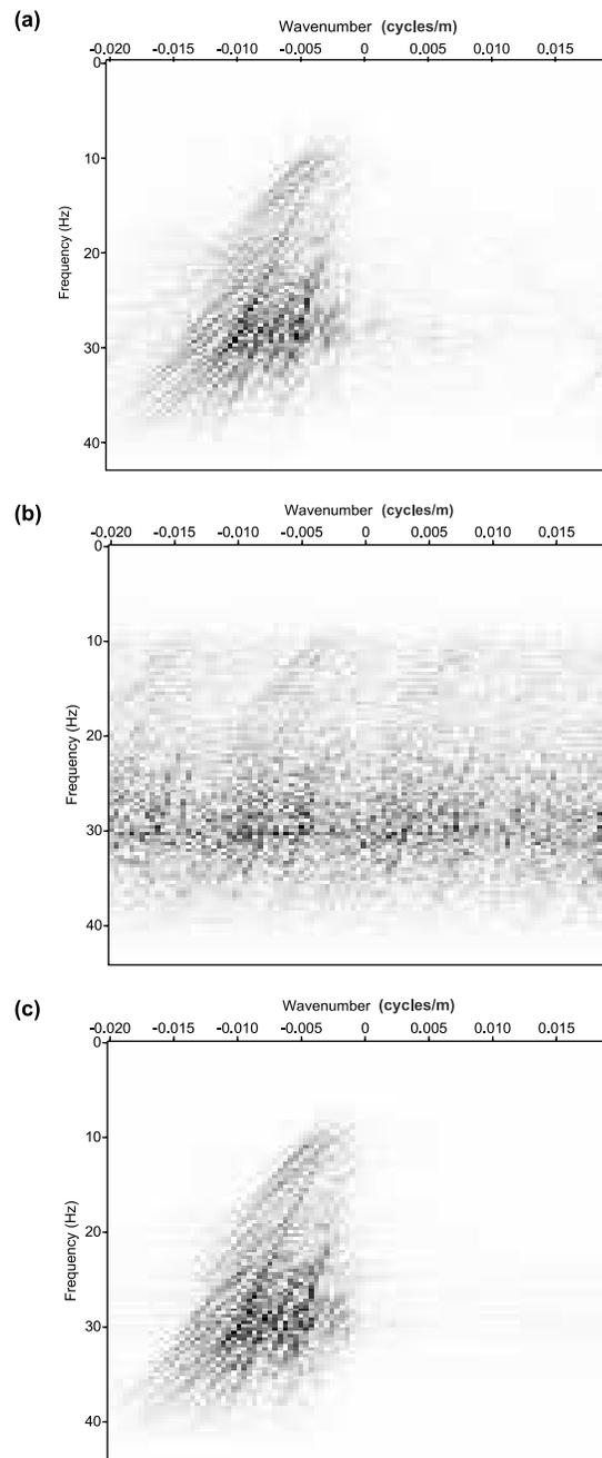
Figure 3.22: (a) The  $f$ - $k$  spectrum of the original shot gather at 3125 m. (b) The  $f$ - $k$  spectrum of the same shot gather after removing 80% traces. (c) The  $f$ - $k$  spectrum of the same shot gather after interpolation.
