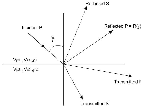
Figure 4.1: Energy partition for a compressional wave (P wave) impinging on a plane interface in an elastic continuum at angle  $\gamma$ . Both reflected and transmitted compressional and shear waves result.
