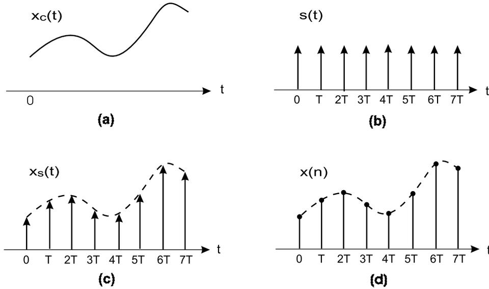
Figure 2.1: The periodic sampling process of a 1-D continuous signal. (a) A continuous signal  $x_c(t)$ . (b) Periodic impulse train  $s(t)$ . (c) The signal  $x_s(t)$ . (d) The discrete sequence  $x(n)$ .
