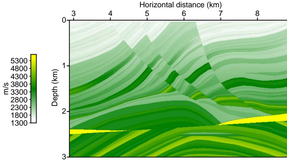
Figure 4.6: The Marmousi compressional velocity field. Velocities range from 1500 to 5500 m/s. The Marmousi model is structurally complex, with many thin layers broken by several major faults and an unconformity surface. The folded carbonate sedimentation series at about 2.5 km form the structural hydrocarbon trap.
