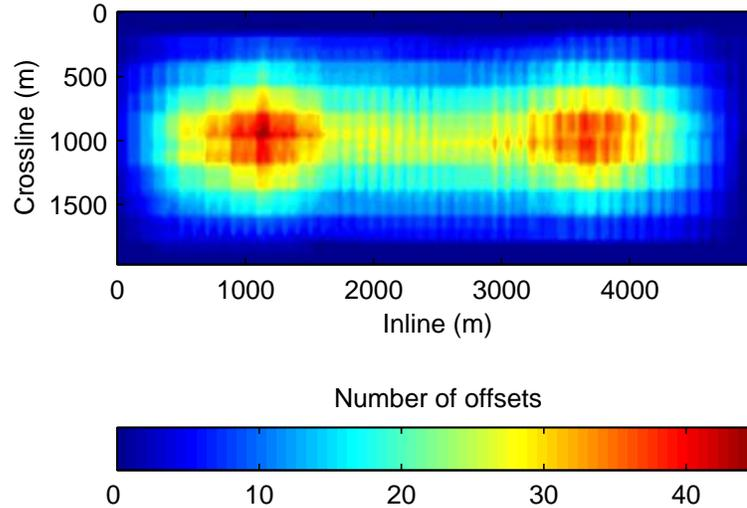
Figure 5.1: Distribution of offsets for the Erskine 3-D data set used to test our interpolation algorithm.
