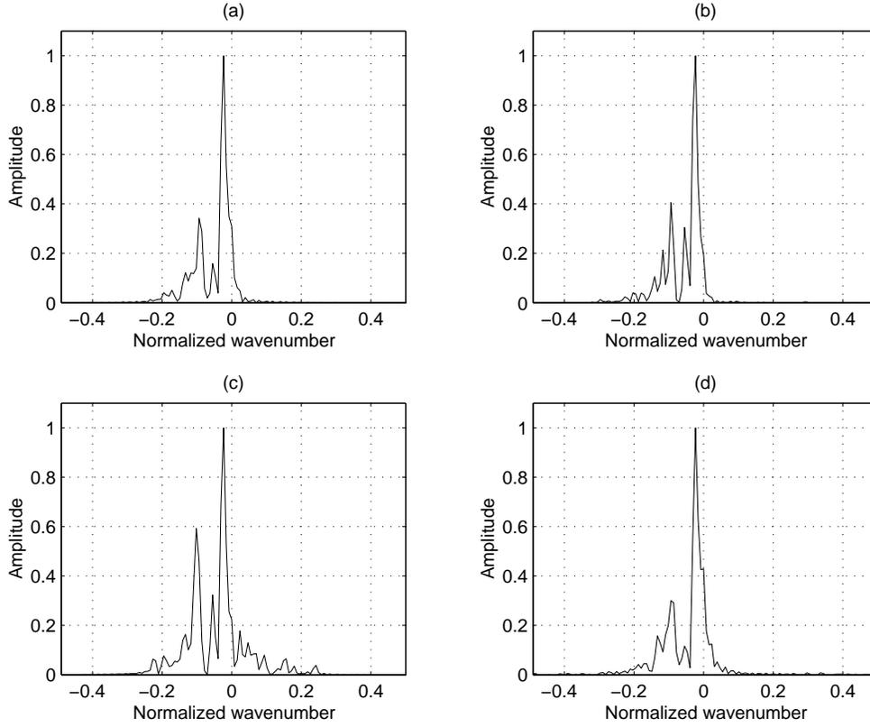
Figure 3.9: Comparison of the reconstructed power spectrum at frequency component  $f = 15.6$  Hz for MWNI, HRFT and MNI Methods. (a) Power spectrum of the reconstructed data using the MWNI method. (b) Power spectrum of the reconstructed data using the HRFT approach. (c) Power spectrum of the reconstructed data using the MNI method. (d) Power spectrum of the original (complete) data.
