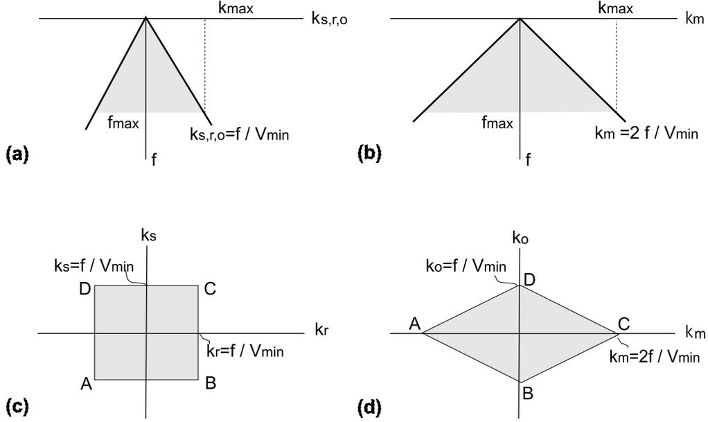
Figure 2.7: (a) Energy distribution in  $(f, k_s)$ ,  $(f, k_r)$  and  $(f, k_o)$ . (b) Energy distribution in  $(f, k_m)$ . (c) Cross-section  $(k_s, k_r)$  of a common frequency panel. (d) Cross-section  $(k_m, k_o)$  of a common frequency panel. Modified after Vermeer (1990).
