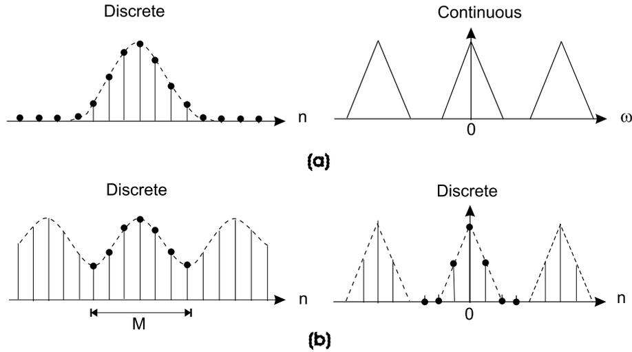
Figure 3.2: (a) An infinite sequence and its discrete time Fourier transform spectrum. (b) A finite sequence and its DFT spectrum.
