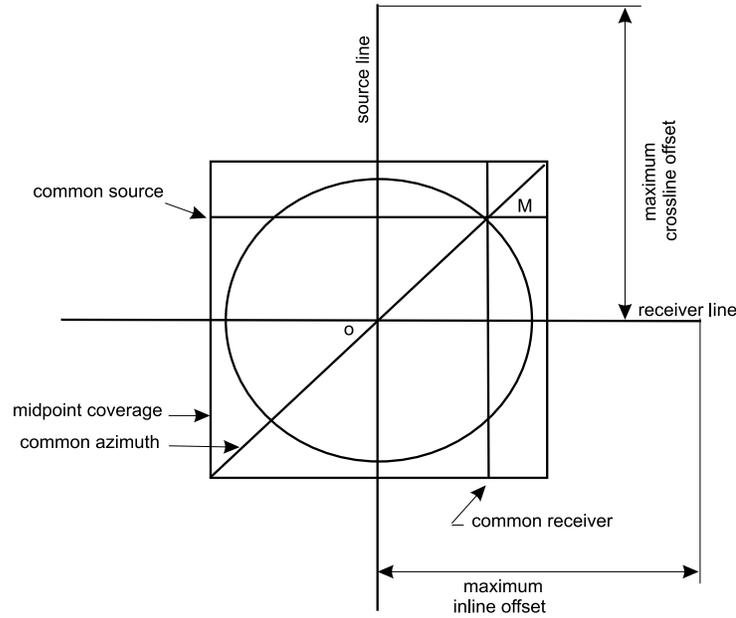
Figure 3.11: Properties of the cross-spread (after Vermeer (1998)). The trace at midpoint  $M$  equals the distance to the center  $O$  of the cross-spread. The trace at  $M$  is a part of a common-source, common-receiver, common offset, and common-azimuth gather.
