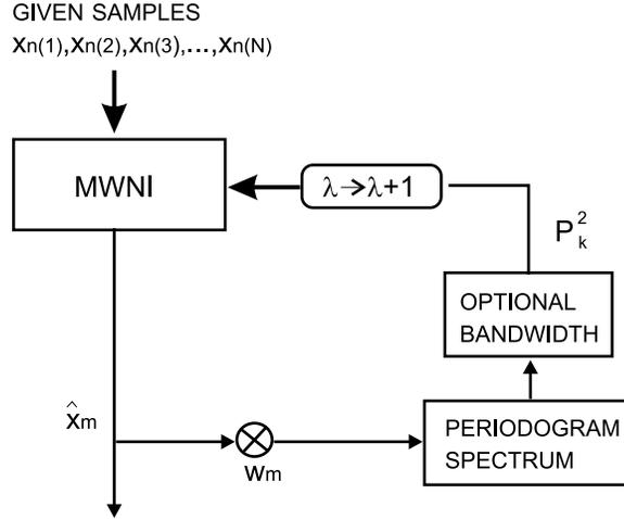
Figure 3.4: Modified periodogram is used to iteratively *bootstrap* the spectral weights from the data.
