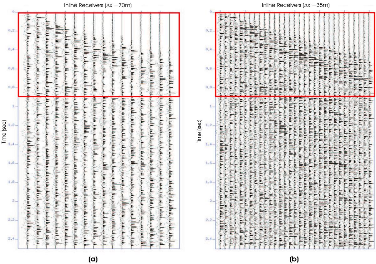
Figure 5.9: Inline receiver interpolation. (a) The original receiver line with a sampling interval of 140 m. (b) The interpolated receiver line with a sampling interval of 35 m.
