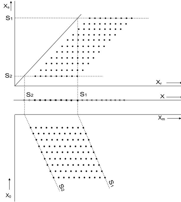
Figure 2.8: Regular off-end shooting geometry, shots moving from right to left. Top:  $(x_s, x_r)$  coordinate system, each dot represents a trace in this system, Middle: Shots and receive  $r$  positions along seismic line, Bottom:  $(x_m, x_o)$  coordinate system, each dot represents a trace in this system. (After Vermeer (1990))
