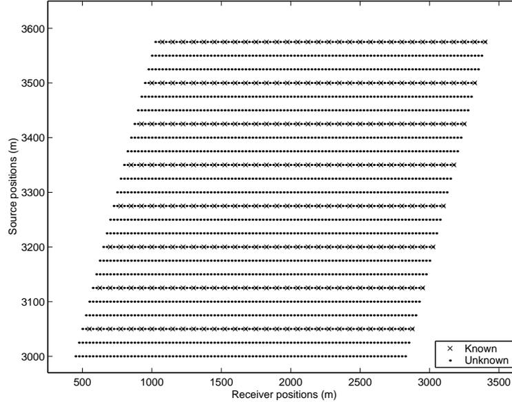
Figure 3.12: Source and receiver position map where the  $\times$ -marks indicate the positions of the available traces; the dots indicate the positions to be interpolated.
