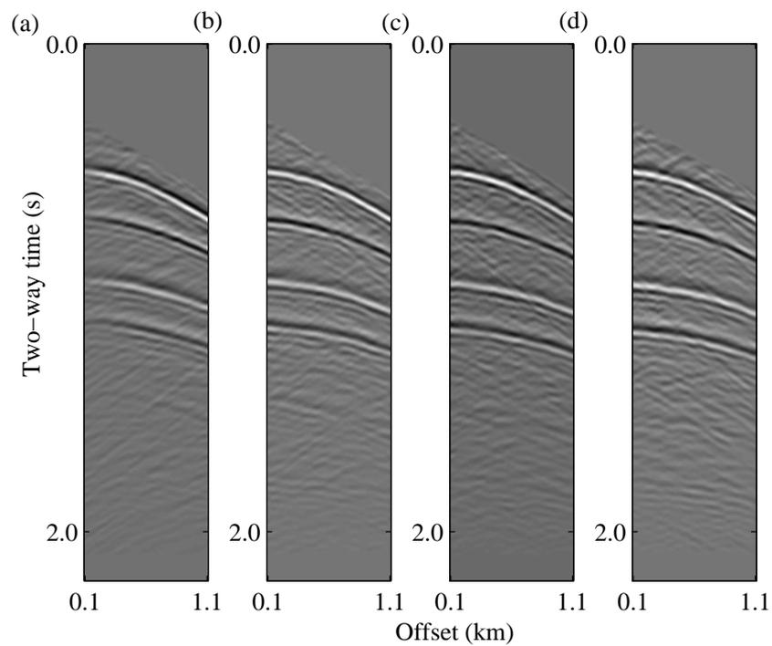
Figure 7.15: Estimated data after 400 model preconditioning based VFSA iterations. (a) Shot location is at the origin (0m, 0m). (b) Shot location is at 300m from the origin. (c) Shot location is at 600m from the origin. (d) Shot location is at 900m from the origin. The search bounds are  $\pm 15\%$  of the true models.
