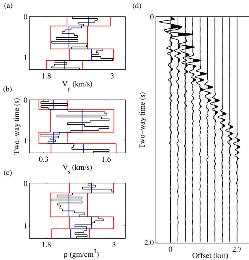
Figure 5.11: The initial model (a)  $V_p$ , (b)  $V_s$ , (c)  $\rho$  and (d) data corresponding to the initial model. The true model is shown in blue line. The upper and lower bounds are shown in red lines and the initial model is shown in black line.
