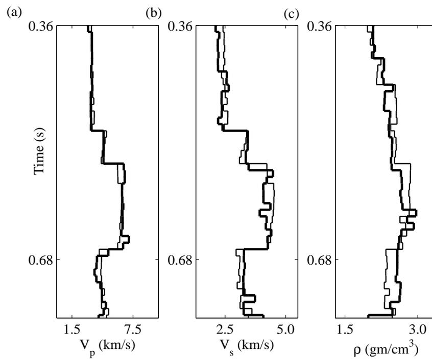
Figure 6.22: The true well log data (thin line) and the estimated well log (thick line). (a) The true and estimated models for  $V_p$ . (b) The true and estimated models for  $V_s$ . (c) The true and estimated models for  $\rho$ . The search bound is  $\pm 25\%$ . The model consists of 50 microlayers of constant time. Total number of unknowns is 150.
