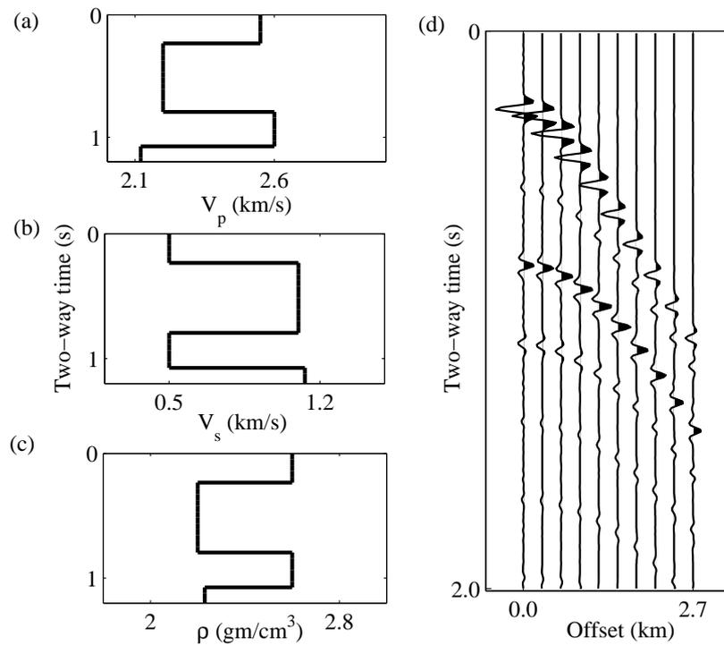
Figure 6.5: The true model and the true synthetic data. (a) The true model for  $\mathbf{V}_p$ . (b) The true model for  $\mathbf{V}_s$ . (c) The true model for  $\rho$ . (d) Synthetic data corresponding to the true model.
