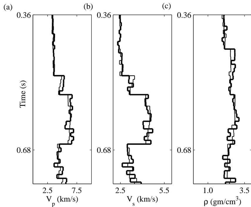
Figure 6.20: The true well log data (thin line) and the estimated well log (thick line). (a) The true and estimated models for  $V_p$ . (b) The true and estimated models for  $V_s$ . (c) The true and estimated models for  $\rho$ . The search bound is  $\pm 15\%$ . The model consists of 50 microlayers of constant time. Total number of unknowns is 150.
