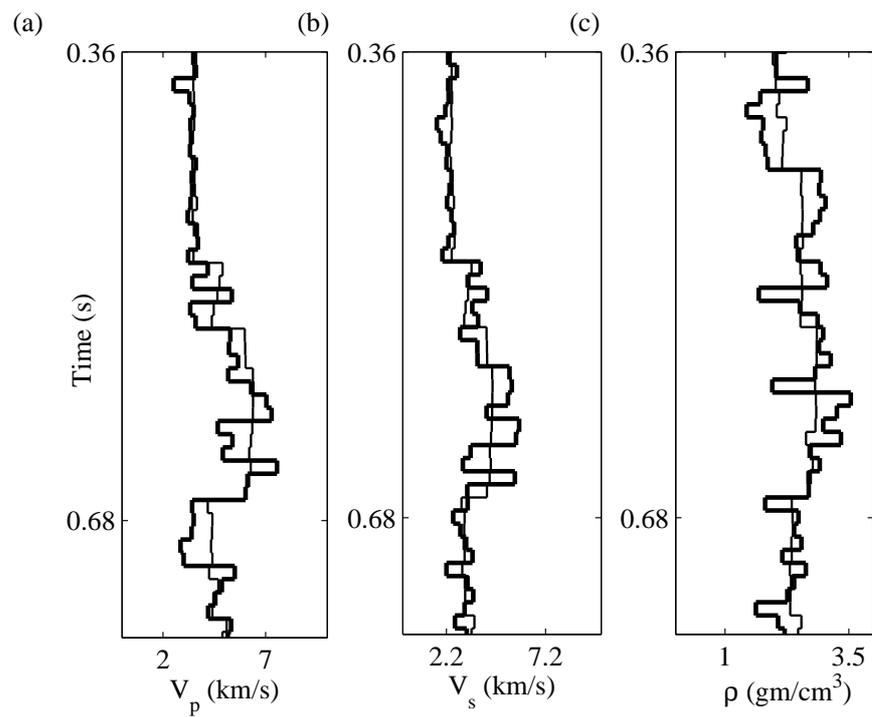
Figure 6.24: The true well log data (thin line) and the estimated well log (thick line). (a) The true and estimated models for  $V_p$ . (b) The true and estimated models for  $V_s$ . (c) The true and estimated models for  $\rho$ . The search bound is  $\pm 35\%$ . The model consists of 50 microlayers of constant time. Total number of unknowns is 150.
