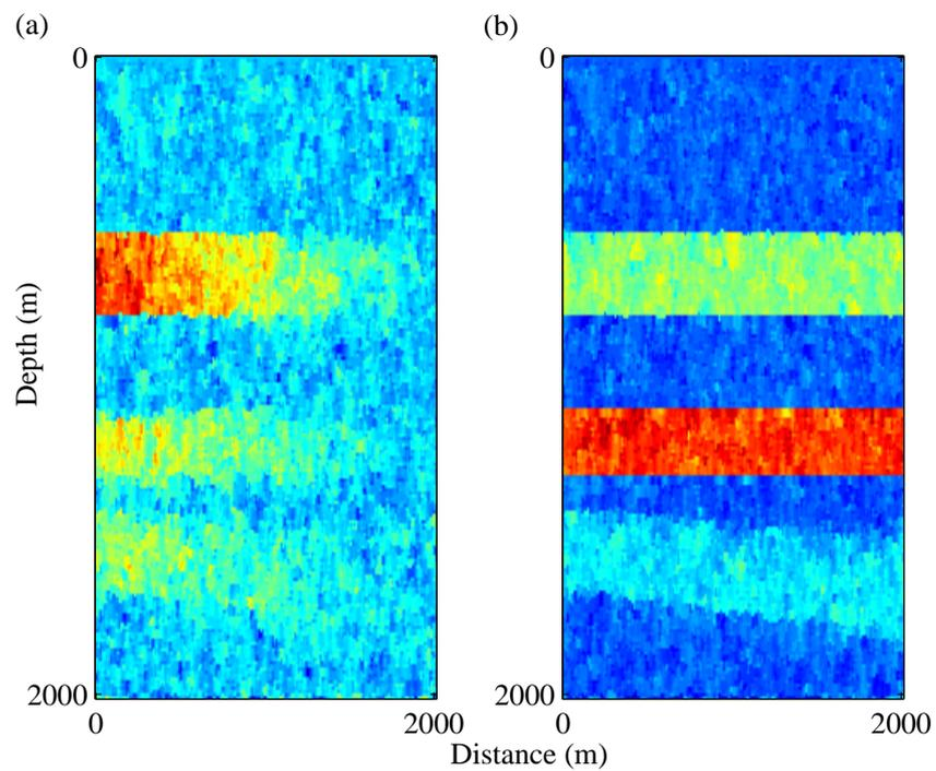
Figure 7.28: Estimated model after 400 model preconditioning based VFSA iterations. (a) Estimated velocity and (b) estimated density. True data contain bandlimited noise such that  $SNR = 10$ . Search bound of the model space is  $\pm 25\%$ .
