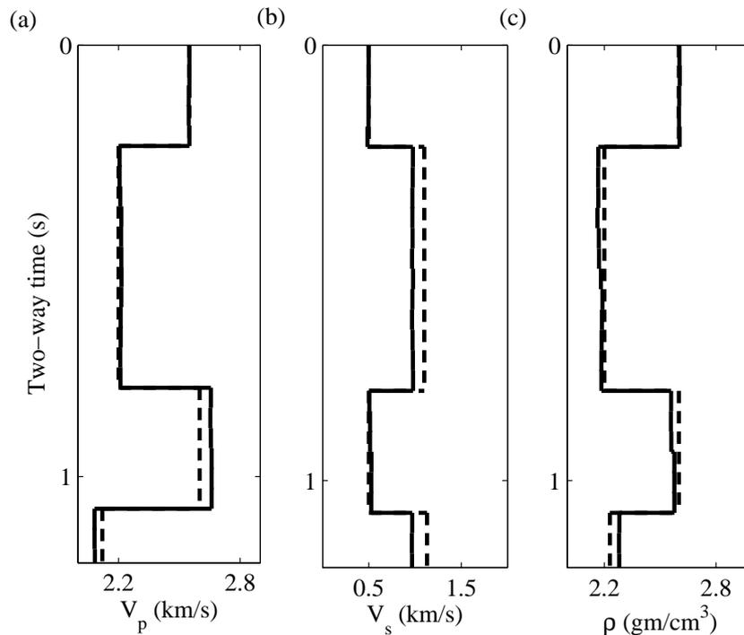
Figure 6.15: Monte Carlo simulations with 100 different random number generating seeds. (a) Mean of 100 Monte Carlo estimations for  $V_p$ . (b) Mean of 100 Monte Carlo estimations for  $V_s$ . (c) Mean of 100 Monte Carlo estimations for  $\rho$ . The solid line represents the estimated profile and the dashed line represents the true profile.
