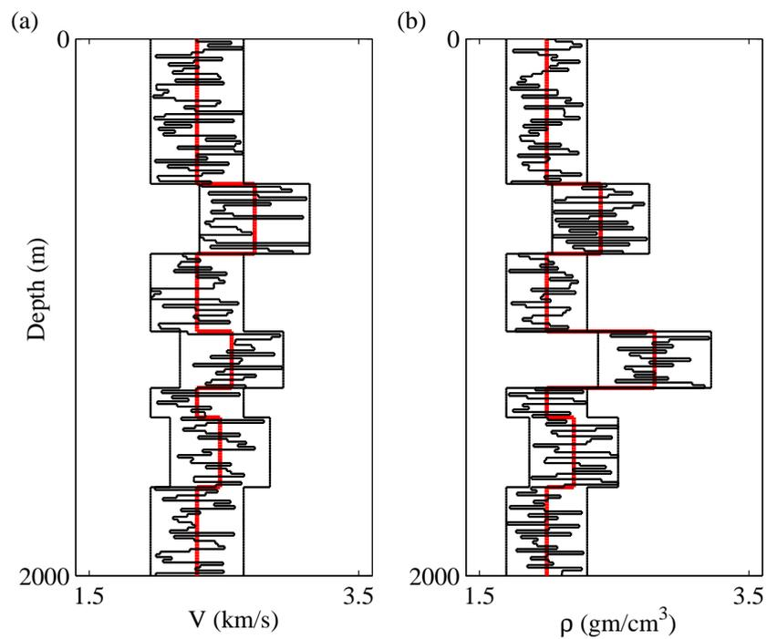
Figure 7.5: The initial velocity and density models in one dimension at the location (300m, 0m). The initial model is chosen with an upper and lower bounds of  $\pm 15\%$  of the respective true values. The red line shows the true model, the blocky line shows the upper and lower bounds of the model space and the zigzag line shows the initial model.
