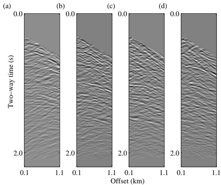
Figure 7.17: Difference between the estimated and the true data. (a) Shot location is at the origin (0m, 0m). (b) Shot location is at 300m from the origin. (c) Shot location is at 600m from the origin. (d) Shot location is at 900m from the origin. The search bounds are  $\pm 15\%$  of the true models.
