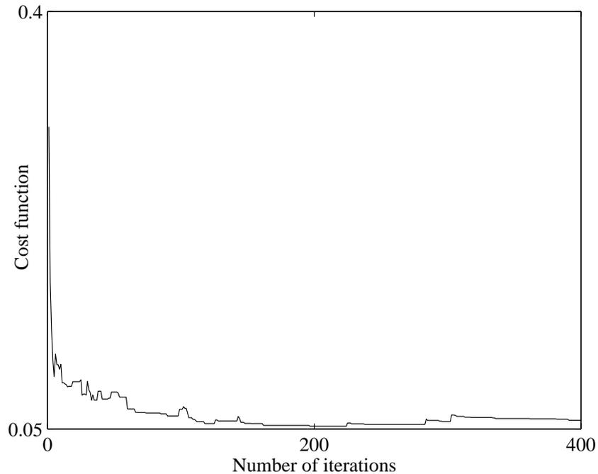
Figure 7.20: The cost function evaluated at each model preconditioning based VFSA optimization. The search bounds are  $\pm 25\%$  of the true models.
