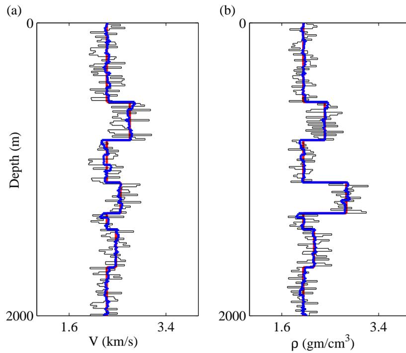
Figure 7.13: Estimated model (blue), true model (red) and initial model (black) for (a) velocity ( $\mathbf{V}$ ) and (b) density ( $\boldsymbol{\rho}$ ). The model search bound is  $\pm 15\%$  of the true model values. Surface location of the vertical profile is 300m from the origin.
