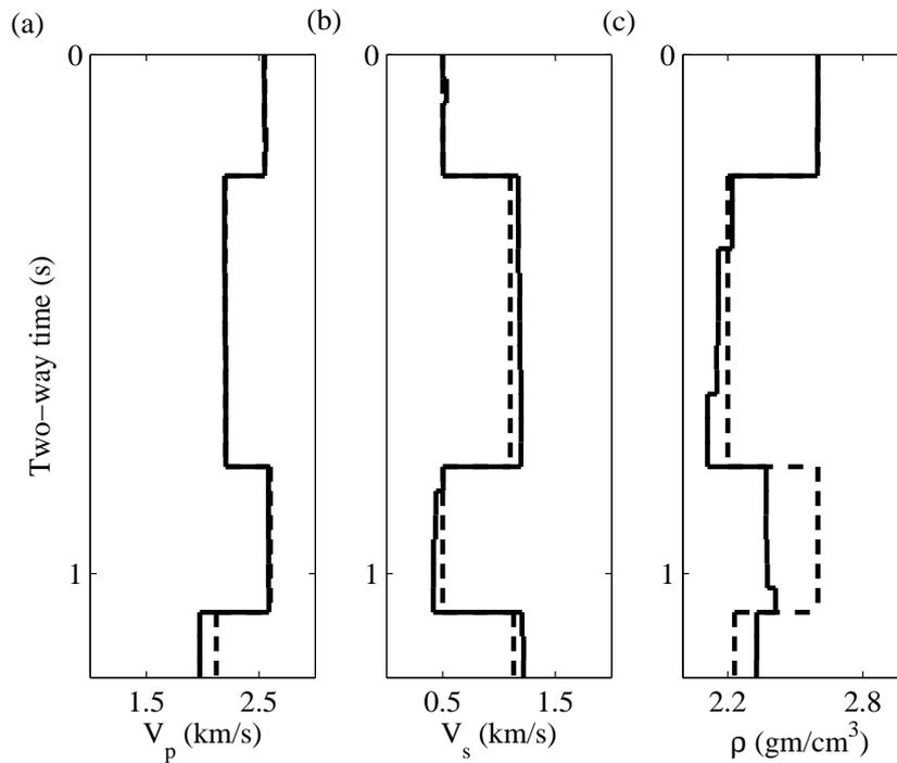
Figure 6.12: (a) Estimated models for  $\mathbf{V}_p$ . (b) The estimated model for  $\mathbf{V}_s$ . (c) The estimated model for  $\rho$ . The solid line shows the estimated model and the dashed line shows the true model. Blocky profiles consistent with the data and *a priori* information are obtained in 6000 evaluations of the forward model in the optimization scheme.
