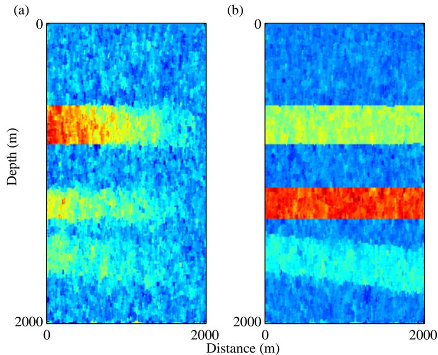
Figure 7.26: Estimated model after 400 model preconditioning based VFSA iterations. (a) Estimated velocity and (b) estimated density. True data contain band-limited noise such that  $SNR = 20$ . Search bound of the model space is  $\pm 25\%$ .
