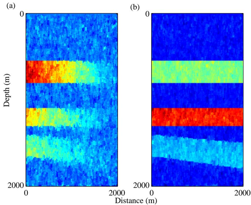
Figure 7.24: Estimated model after 400 model preconditioning based VFSA iterations. (a) Estimated velocity and (b) estimated density. True data contain band-limited noise such that  $SNR = 10$ . Search bound of the model space is  $\pm 15\%$ .
