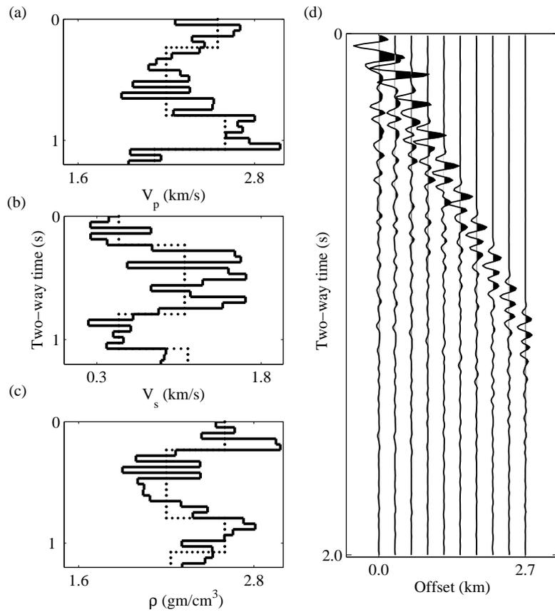
Figure 6.6: The random initial model and the synthetic data corresponding to the initial model. (a) The initial model for  $V_p$ . (b) The initial model for  $V_s$ . (c) The initial model for  $\rho$ . The solid line shows the initial model and the dotted line shows the true model. (d) The synthetic data corresponding to the initial model. The figure shows that the starting model is not close to the global minimum of the cost function topology.
