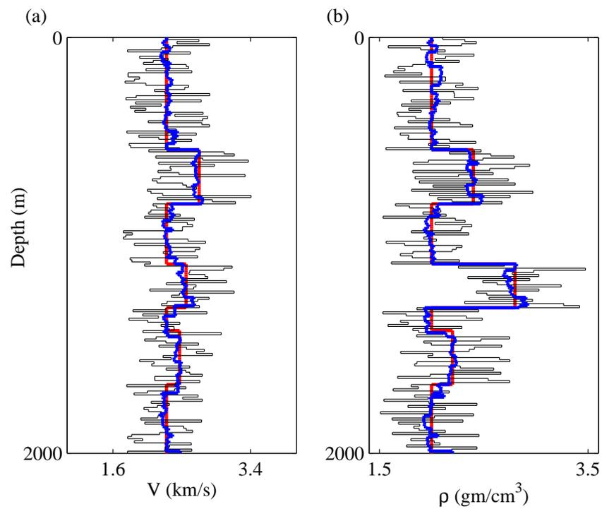
Figure 7.14: Estimated model (blue), true model (red) and initial model (black) for (a) velocity ( $\mathbf{V}$ ) and (b) density ( $\rho$ ). The model search bound is  $\pm 25\%$  of the true model values. Surface location of the vertical profile is 300m from the origin.
