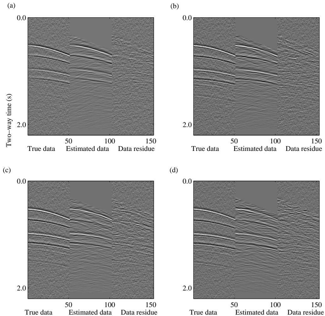
Figure 7.27: True data, estimated data and data residue. (a) Shot location is at the origin (0m,0m). (b) Shot location is at 300m from the origin. (c) Shot location is at 600m from the origin. (d) Shot location is at 900m from the origin. True data contain bandlimited noise such that  $SNR = 10$ . Search bound of the model space is  $\pm 25\%$ .
