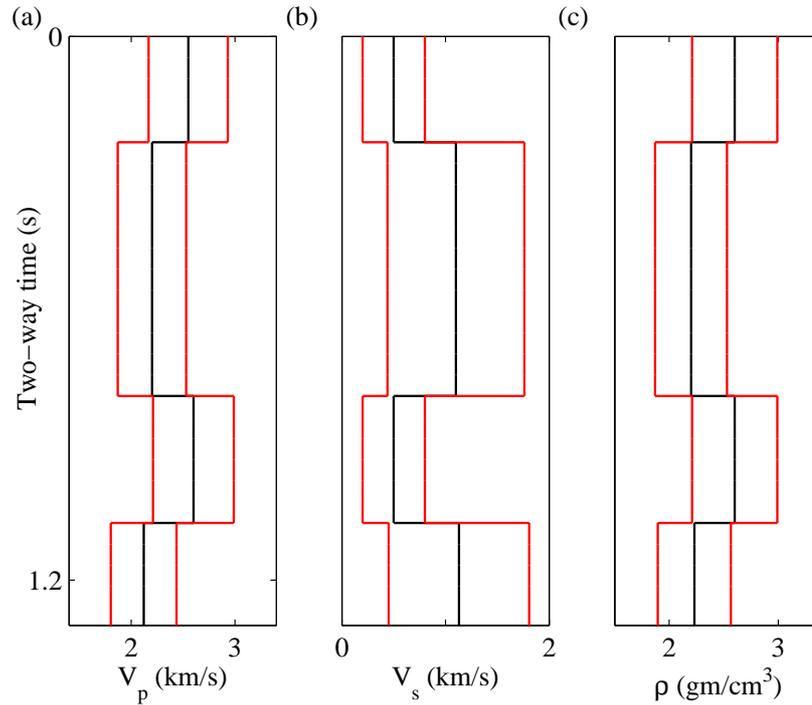
Figure 6.4: The upper and lower bounds of the model space. (a) The bounds for  $\mathbf{V}_p$ . (b) The bounds for  $\mathbf{V}_s$ . (c) The bounds for  $\rho$ . The black line shows the true model value and the red line shows the upper and lower bounds. The bounds are  $\pm 15\%$  for  $\mathbf{V}_p$  and  $\rho$  and  $\pm 60\%$  for  $\mathbf{V}_s$  with respect to the true model.
