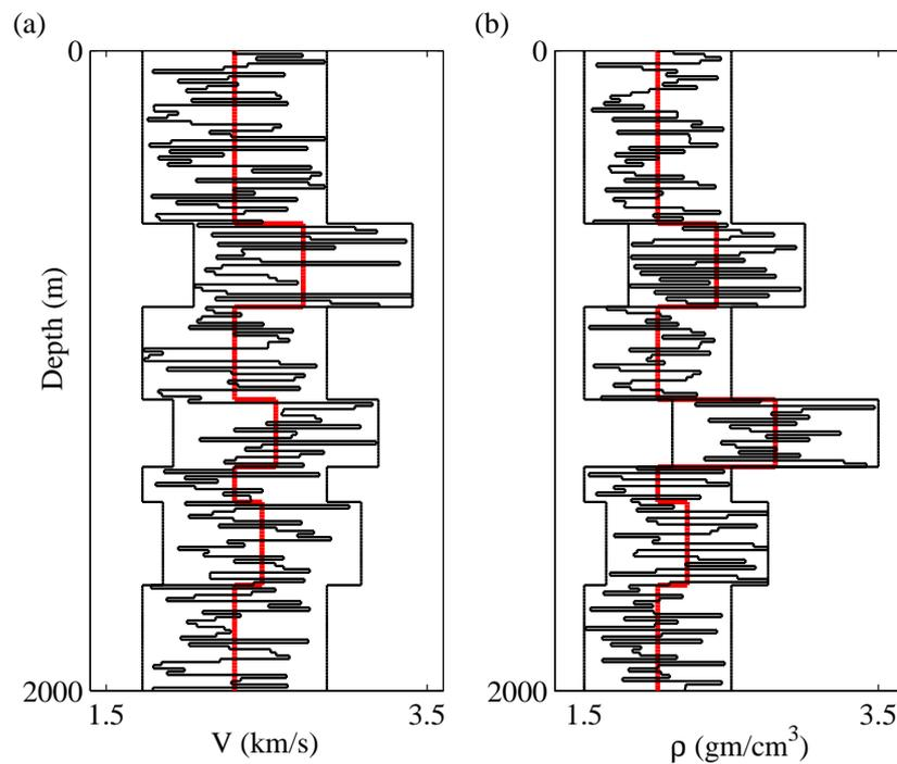
Figure 7.6: The initial velocity and density models in one dimension at the location (300m, 0m). The initial model is chosen with an upper and lower bounds of  $\pm 25\%$  of the respective true values. The red line shows the true model, the blocky line shows the upper and lower bounds of the model space and the zigzag line shows the initial model.
