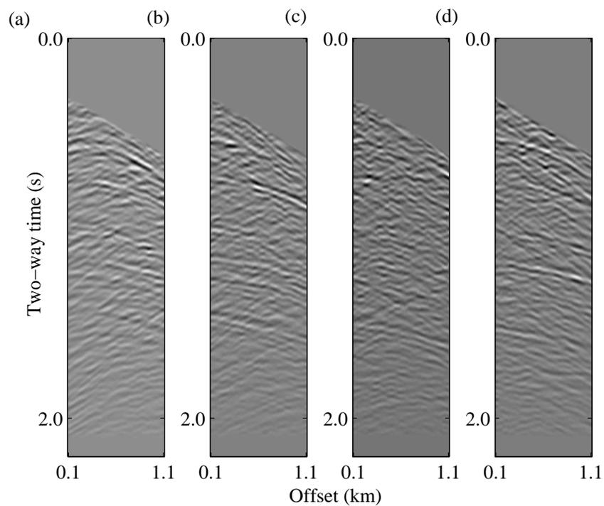
Figure 7.18: Difference between the estimated and the true data. (a) Shot location is at the origin (0m, 0m). (b) Shot location is at 300m from the origin. (c) Shot location is at 600m from the origin. (d) Shot location is at 900m from the origin. The search bounds are  $\pm 25\%$  of the true models.
