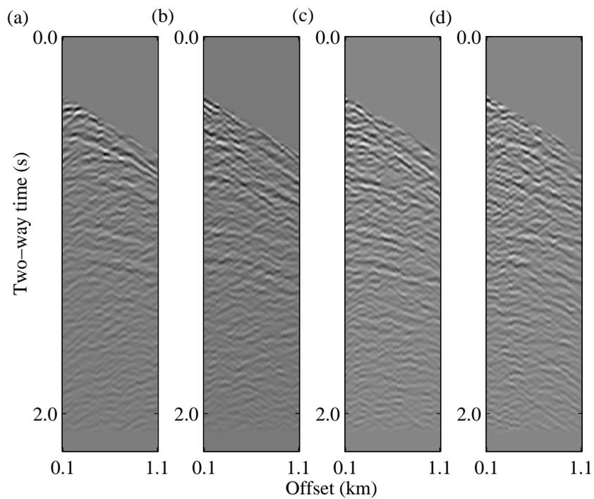
Figure 7.8: Data corresponding to the initial model chosen within  $\pm 25\%$  bounds of the true model. (a) Shot location at the origin (0m,0m). (b) Shot location at 300m from the origin. (c) Shot location at 600m from the origin and (d) Shot location at 900m from the origin.
