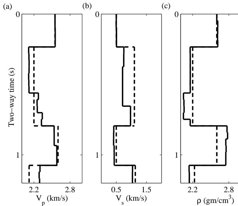
Figure 6.14: (a) Estimated models for  $V_p$ . (b) The estimated model for  $V_s$ . (c) The estimated model for  $\rho$ . The solid line shows the estimated model and the dashed line shows the true model. Blocky profiles consistent with the data and *a priori* information are obtained in 6000 evaluations of the forward model in the optimization scheme.
