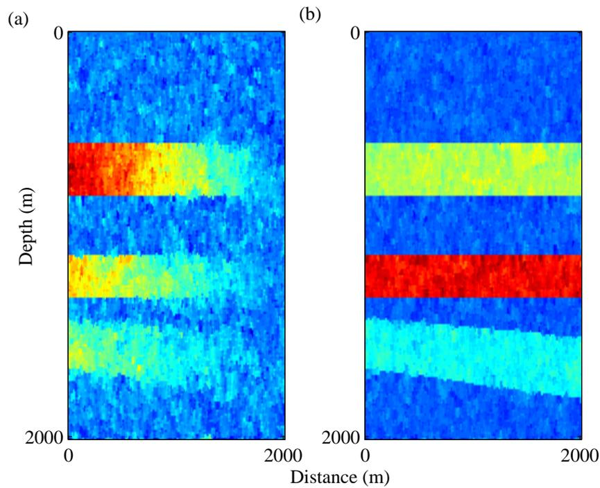
Figure 7.22: Estimated model after 400 model preconditioning based VFSA iterations. (a) Estimated velocity and (b) estimated density. True data contain band-limited noise such that  $SNR = 20$ . Search bound of the model space is  $\pm 15\%$ .
