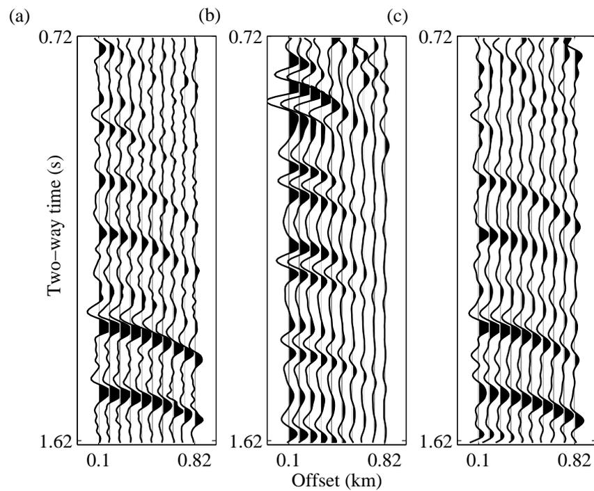
Figure 6.23: (a) The true well log simulated data with bandlimited noise. (b) The data corresponding to the initial model. (c) The estimated data obtained by the model preconditioning based very fast simulated annealing optimization algorithm. The model search space is  $\pm 35\%$  of the true well log data.
