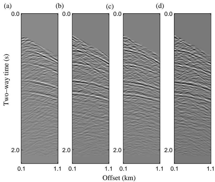
Figure 7.9: Difference between data corresponding to the initial model chosen within  $\pm 15\%$  bounds of the true model and the true data. (a) Shot location at the origin (0m, 0m). (b) Shot location at 300m from the origin. (c) Shot location at 600m from the origin and (d) Shot location at 900m from the origin.
