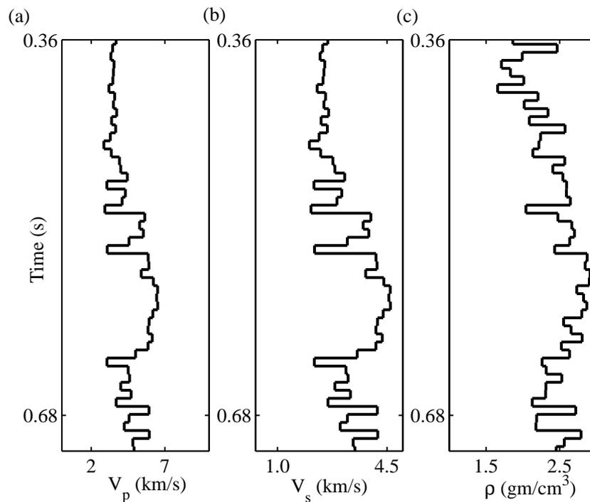
Figure 6.17: The well log data. (a) The well log data for  $V_p$ . (b) The well log data for  $V_s$ . (c) The well log data for  $\rho$ . The S-wave well log is synthetically generated from the P-wave well log.
