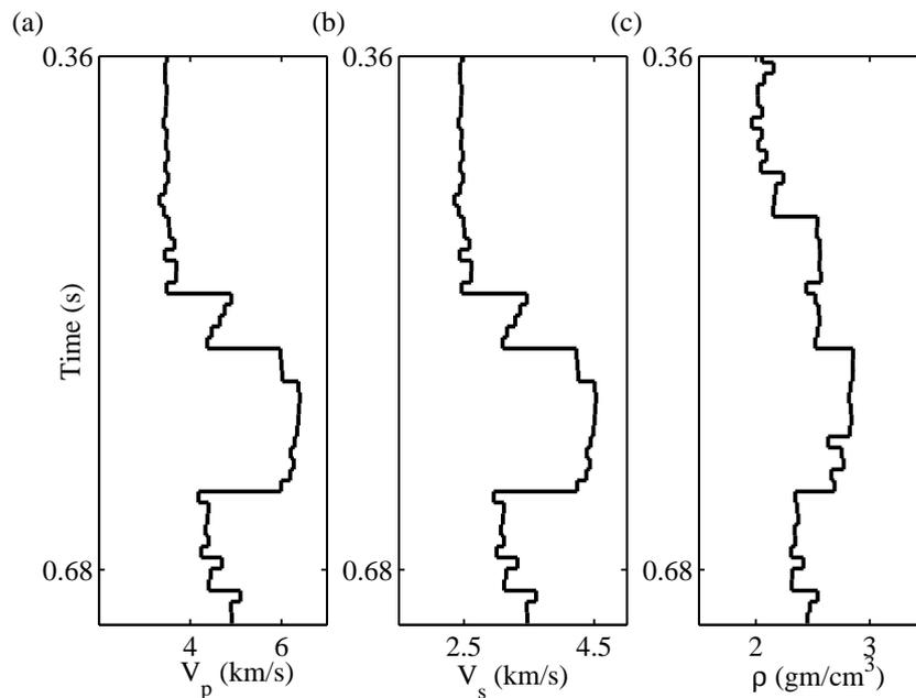
Figure 6.18: Well log data after application of EPS filter. It is observed that the EPS filter enhanced the edgy features in the profiles while suppressing the high frequency fluctuations that are not ordinarily represented in the data.
