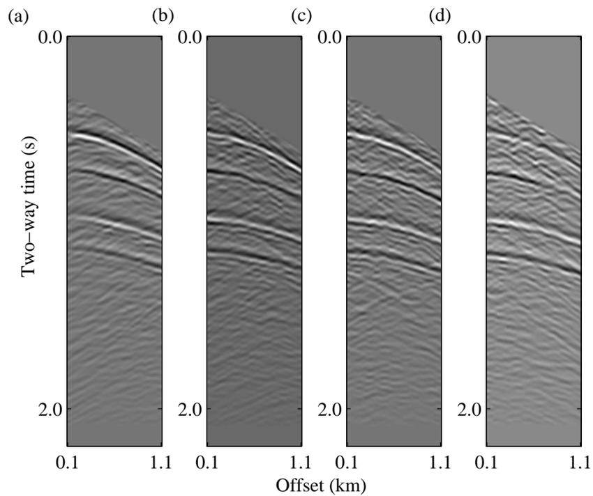
Figure 7.16: Estimated data after 400 model preconditioning based VFSA iterations. (a) Shot location is at the origin (0m,0m). (b) Shot location is at 300m from the origin. (c) Shot location is at 600m from the origin. (d) Shot location is at 900m from the origin. The search bounds are  $\pm 25\%$  of the true models.
