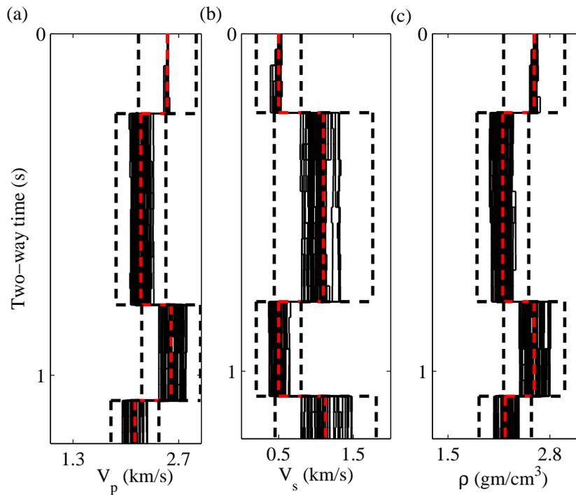
Figure 6.16: Monte Carlo simulations showing estimated models within  $\pm 50\%$  of the search bounds. A total of 100 Monte Carlo simulations was performed. (a) Estimations for  $\mathbf{V}_p$  (46 numbers). (b) Estimations for  $\mathbf{V}_s$  (46 numbers). (c) Estimations for  $\rho$  (49 numbers). The outer dashed lines represent the search bounds.
