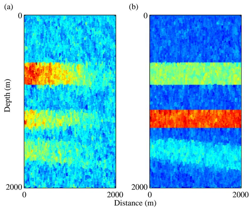
Figure 7.12: Estimated velocity and density model after 400 model preconditioning based VFSA iterations. (a) The estimated velocity model and (b) the estimated density model. The model search bound is  $\pm 25\%$  of the true model values.
