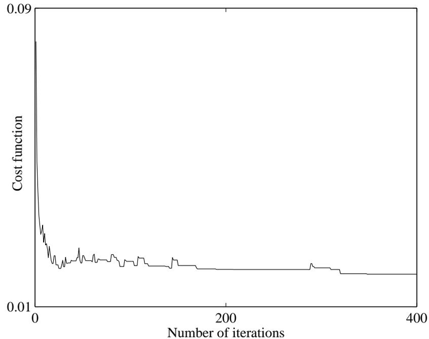
Figure 7.19: The cost function evaluated at each model preconditioning based VFSA optimization. The search bounds are  $\pm 15\%$  of the true models.
